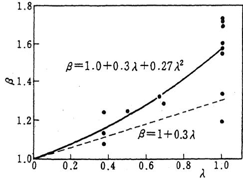
Fig. 6 : Shear strength magnification by transverse beams
