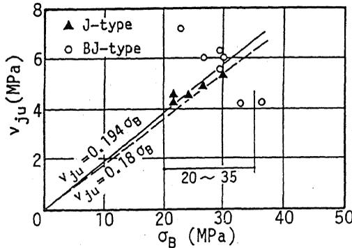
Fig. 5 : Average shear stress-concrete strength (exterior joint)
