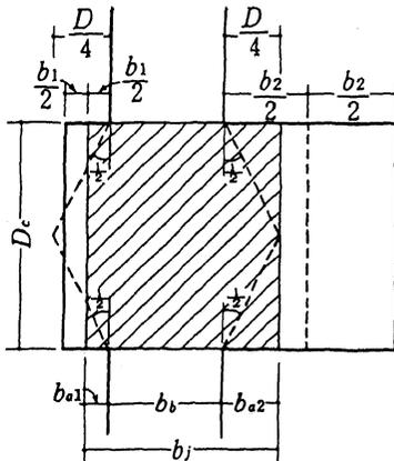
Fig. 3 : Effective width of beam-column joint
