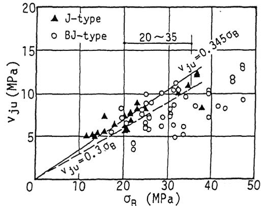
Fig. 4 : Average shear stress-concrete strength (interior joint)
