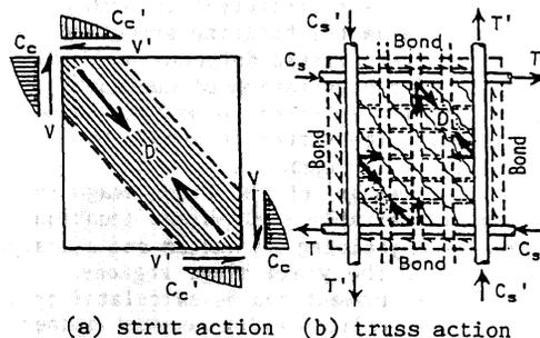
(a) strut action (b) truss action
