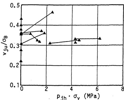
Fig. 8 : Effect of lateral reinforcement in interior joint
