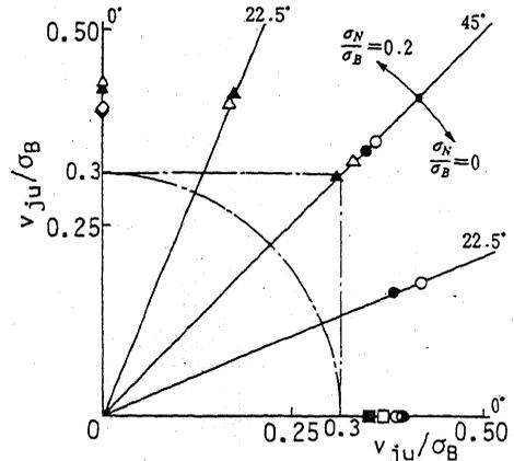
Fig. 7 : Bi-directional Shear Interaction
