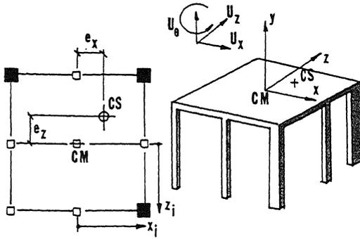
Fig. 1 Single story structure model
