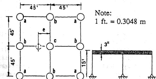
Fig. 2 Column plan of study models
