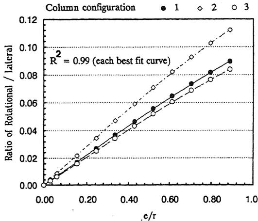
Fig. 3 Best fit curve for torsional to coupled lateral response as a function of normalized eccentricity
