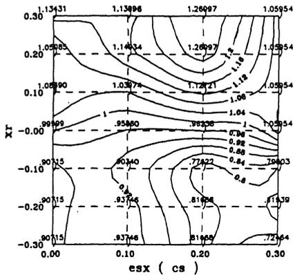
Fig. 5. Envelope of maximum ductility ratio versus  $e_s$  and  $X_R$ . Design 1,  $T_x=T_y=1.5$  sec,  $Q=4$ ,  $h/b=1$ .
