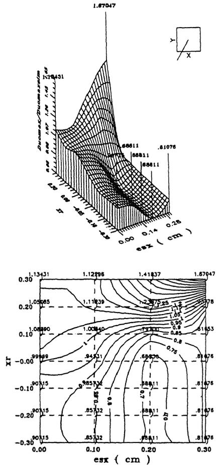
Fig. 4. Envelope of maximum ductility ratio versus  $e_x$  and  $X_R$ . Design 1,  $T_x=T_y=1.5$  sec,  $Q=4$ ,  $h/b=1.0$ .
