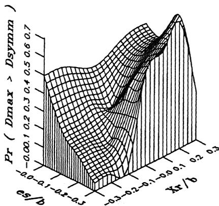
Fig. 8. Probability of exceedence of the maximum ductility demand versus  $e$ , and  $X_R$ . Design 1,  $T=1.0$  sec,  $Q=4$ ,  $h/b=1$ , one direction.
