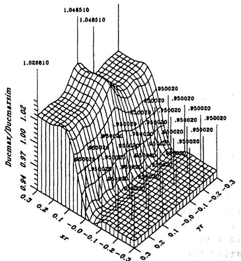
Fig.7. Envelope of max. duc. ratio versus  $X_R$  and  $Y_R$ .  $e_s=0.3b$ , Designs 1-3,  $T=1.5$  s,  $Q=4$ ,  $h/b=1$ , 2 direc.
