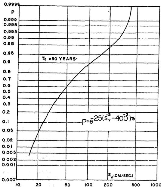
Figure 2. Accumulated probability distribution,  $P$ , of the maximum values of the pseudovelocity spectra,  $S_v(10\%)$ , for a lapse time period of 50 years, for Mexico City Lake zone.
