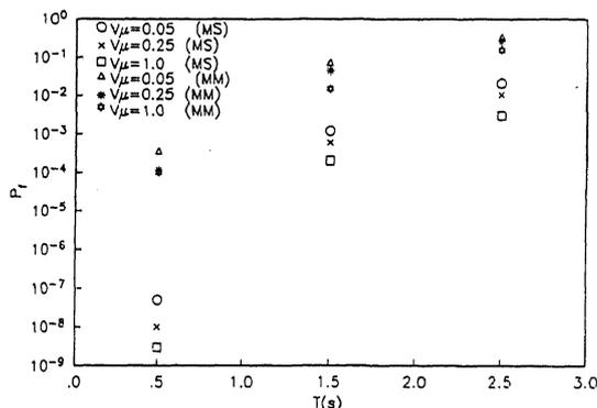
Figure 7. Probability of failure,  $P_f$ , for single frame (MS) and single infilled frame, (MM), systems designed according with Mexico's City 1987 Construction Code, with initial natural periods of 0.5, 1.5, and 2.5s. A nominal ductility factor  $\mu = 4$  is assumed, for coefficients of variation  $V_\mu = 0.05, 0.25$ , and 1. The systems are assumed to be located on Mexico's City Lake zone.
