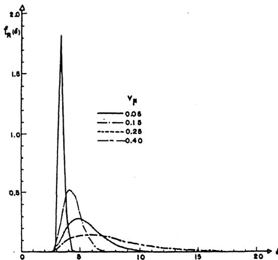
Figure 6. Probability density function,  $f_R$ , of the nominal ductility,  $\mu = 4$ , assumed for the single frame and the single infilled frame; the  $f_R$  is shown for several coefficients of variation,  $V_\mu$ , and  $\delta = \mu - 1$ .
