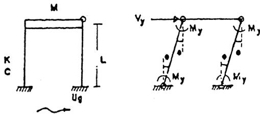
Figure 3. Single frame system and its collapse mechanism.
