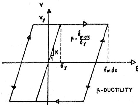
Figure 5. Idealized elastoplastic hysteretic behaviour of the single frame and single infilled frame system.
