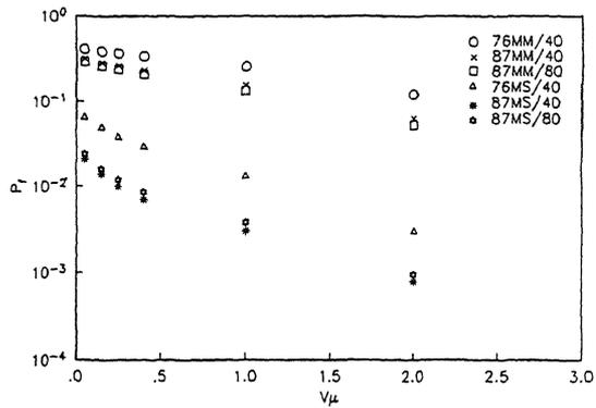
Figure 8 . Variation of the probability of failure,  $P_f$ , with  $V\mu$ , for single frame, (MS), and single infilled frame, (MM), structural systems, designed according with Mexico's City 1976, (76), and 1987, (87), Construction Codes. An initial natural period of 2.5s is assumed for both systems. Families of 40 and 80 structural systems were used in the Monte Carlo simulation. See Figure 7 for complementary information.
