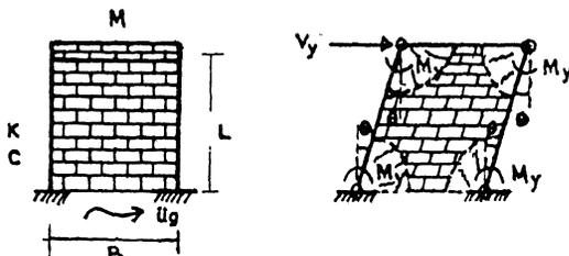
Figure 4. Single infilled frame system and its collapse mechanism.
