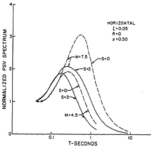
Fig. 1 Normalized PSV spectra for magnitudes  $M = 4.5$  and  $7.5$ , for probability of exceedance  $p = 0.5$ , fraction of critical damping  $\zeta = 0.05$ , at zero epicentral distances,  $R = 0$ , on basement rock ( $s = 2$ ) and on sediments ( $s = 0$ ) (after Trifunac, 1978).
