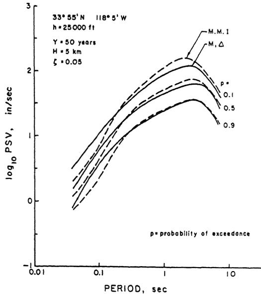
Fig. 5 Uniform risk spectrum at site 33° 55' N, 118° 5' W, with thickness of sediments  $h = 25000$  ft, for surrounding sources at depth  $H = 5$  km, fraction of critical damping  $\zeta = 0.05$  and for exposure time of 50 years. Dashed lines show URS amplitudes computed via MMI, and solid lines for amplitude attenuation in terms of magnitude  $M$ , and hypocentral distance  $\Delta$ .
