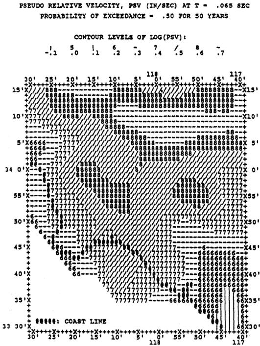
Fig. 4 Microzonation map for PSV amplitudes at  $T = .065$  sec, with probability of exceedance  $p = 0.5$ , during exposure time of 50 years.
