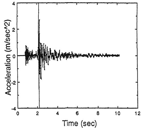
Fig. 3 Tennant Creek earthquake aftershock accelerogram
