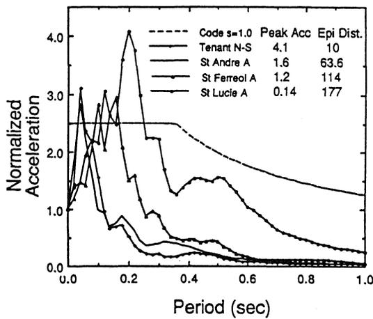
Fig. 2.1 Intraplate earthquake and design response spectra
