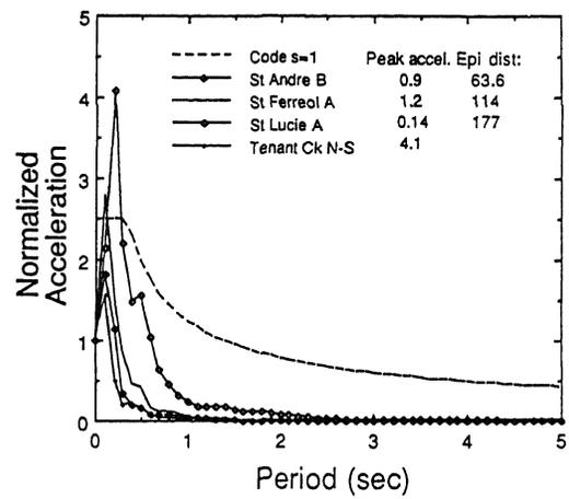
Fig. 2.2 Intraplate earthquake and design response spectra
