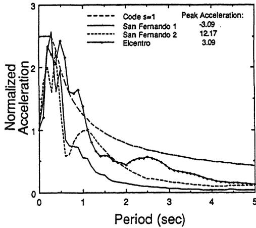
Figure 1 Interplate earthquake and design response spectra
