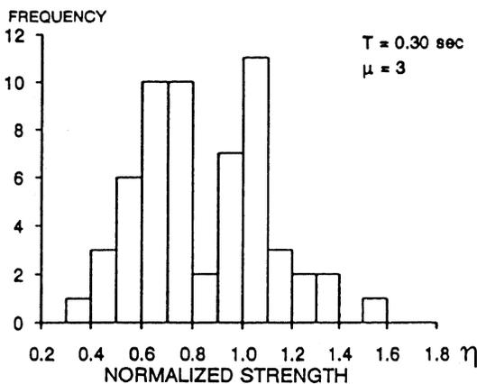
Figure 7. Frequency histogram of normalized strength demands for alluvium sites ( $T=0.4$  sec and  $\mu=3$ ).
