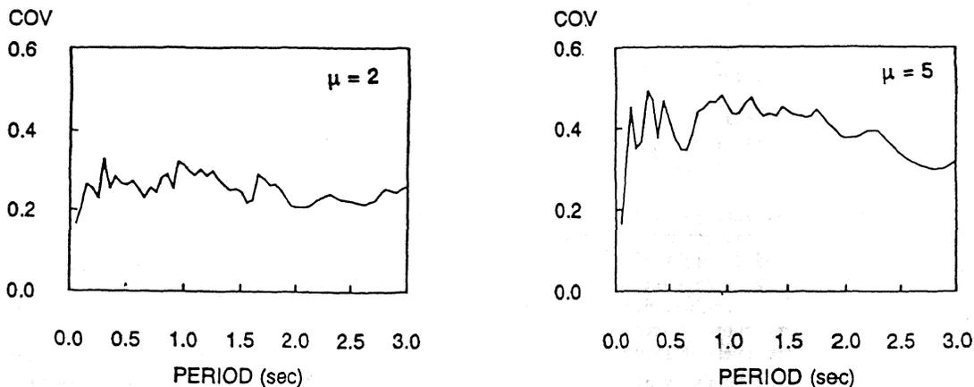
Figure 5. Coefficients of variation of strength reduction factors for alluvium sites and ductilities of 2 and 5.
