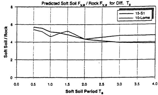
Figure 14. Variation of maximum amplification of elastic strength demand with  $T_s$  and record set
