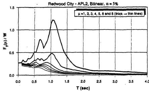
Figure 3. Elastic and inelastic strength demand spectra for APL2 soft soil record
