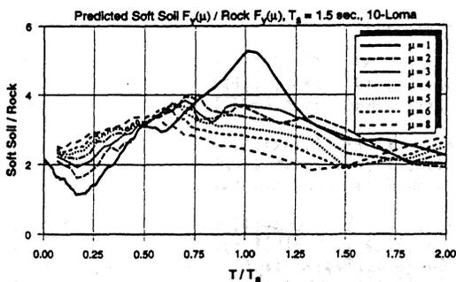
Figure 13. Mean amplifications of elastic and inelastic strength demands for  $T_s = 1.5$  sec., 10-Loma record set
