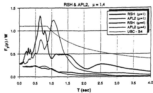
Figure 5. Elastic and inelastic strength demand spectra for two recorded soft soil motions
