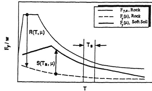
Figure 17. Suggested process for modification of SDOF strength demands for soft soil effects
