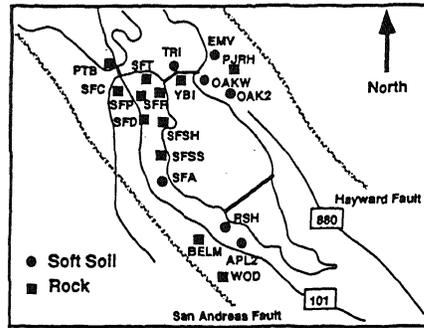
Figure 2. Locations of Loma Prieta ground motion stations used in this study
