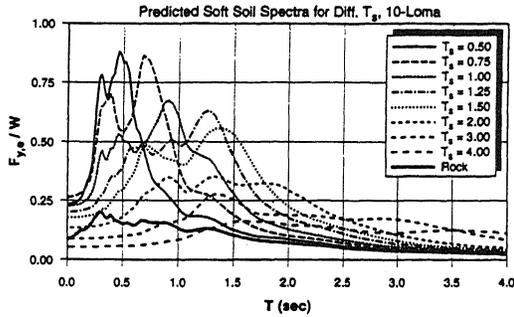
Figure 10. Mean elastic strength demand spectra for soft soil and rock motions, 10-Loma record set
