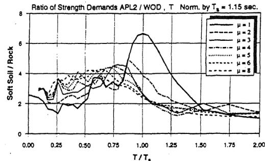
Figure 6. Amplification of strength demands obtained from a pair of nearby soft soil and rock records
