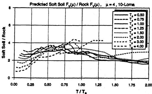
Figure 12. Mean amplification of inelastic strength demands for  $\mu = 4$ , 10-Loma record set
