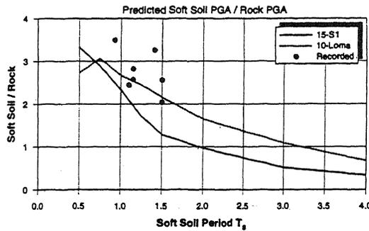
Figure 16. Mean amplifications of PGA computed from 15-S<sub>1</sub> and 10-Loma record sets
