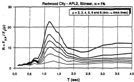
Figure 4. Strength reduction factors for APL2 soft soil record
