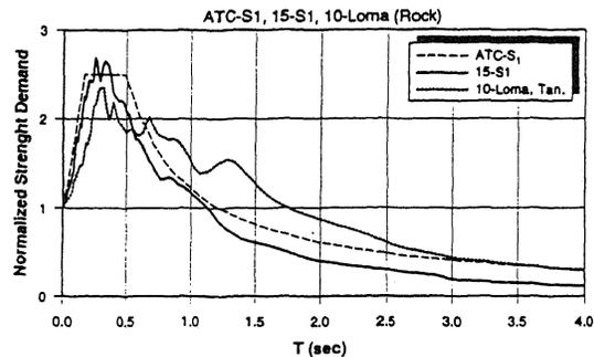
Figure 9. Means of normalized elastic spectra of 15-S1 and 10-Loma rock records
