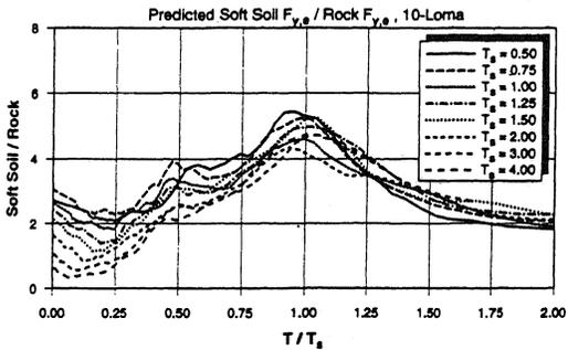
Figure 11. Mean amplification of elastic strength demands, 10-Loma record set
