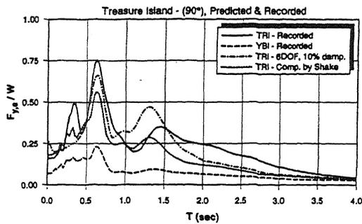
Figure 7. Elastic strength demand spectra obtained from recorded and predicted soft soil motions
