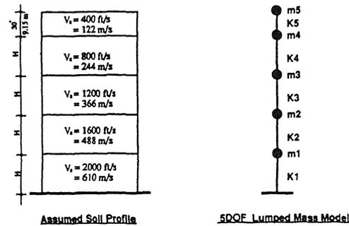
Figure 8. Soil column models used in parameter study
