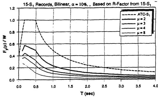
Figure 1. Inelastic strength demand spectra based on ATC  $S_1$  ground motion spectrum
