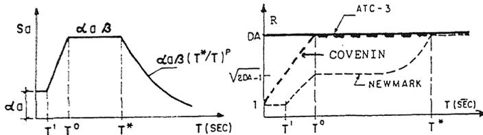
Figure 1. Elastic spectrum  $S_a$  and Reduction Factor  $R$ ; typical code shapes.
