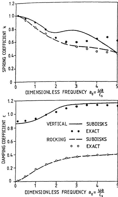
Figure 7. Dynamic-stiffness coefficients of square foundation on soil halfspace ( $\nu = 1/3$ ).
