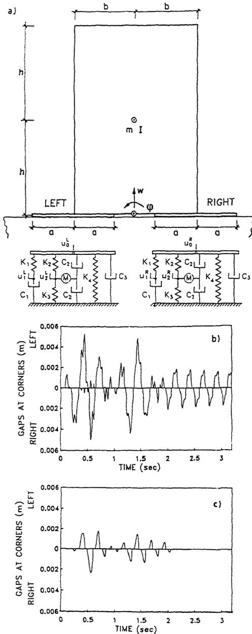
Figure 13. Rigid block on layer and halfspace with partial uplift.
