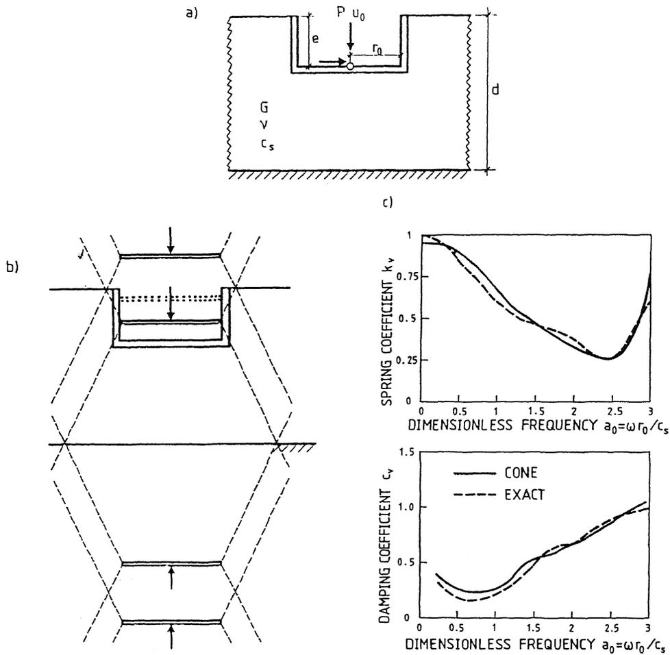
Figure 3. Vertical motion of foundation embedded in soil layer on rigid rock.
