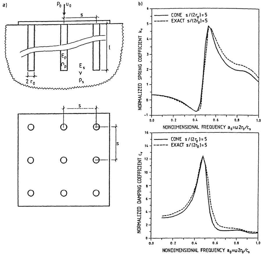
Figure 8. Vertical motion of floating pile group in soil halfspace.
