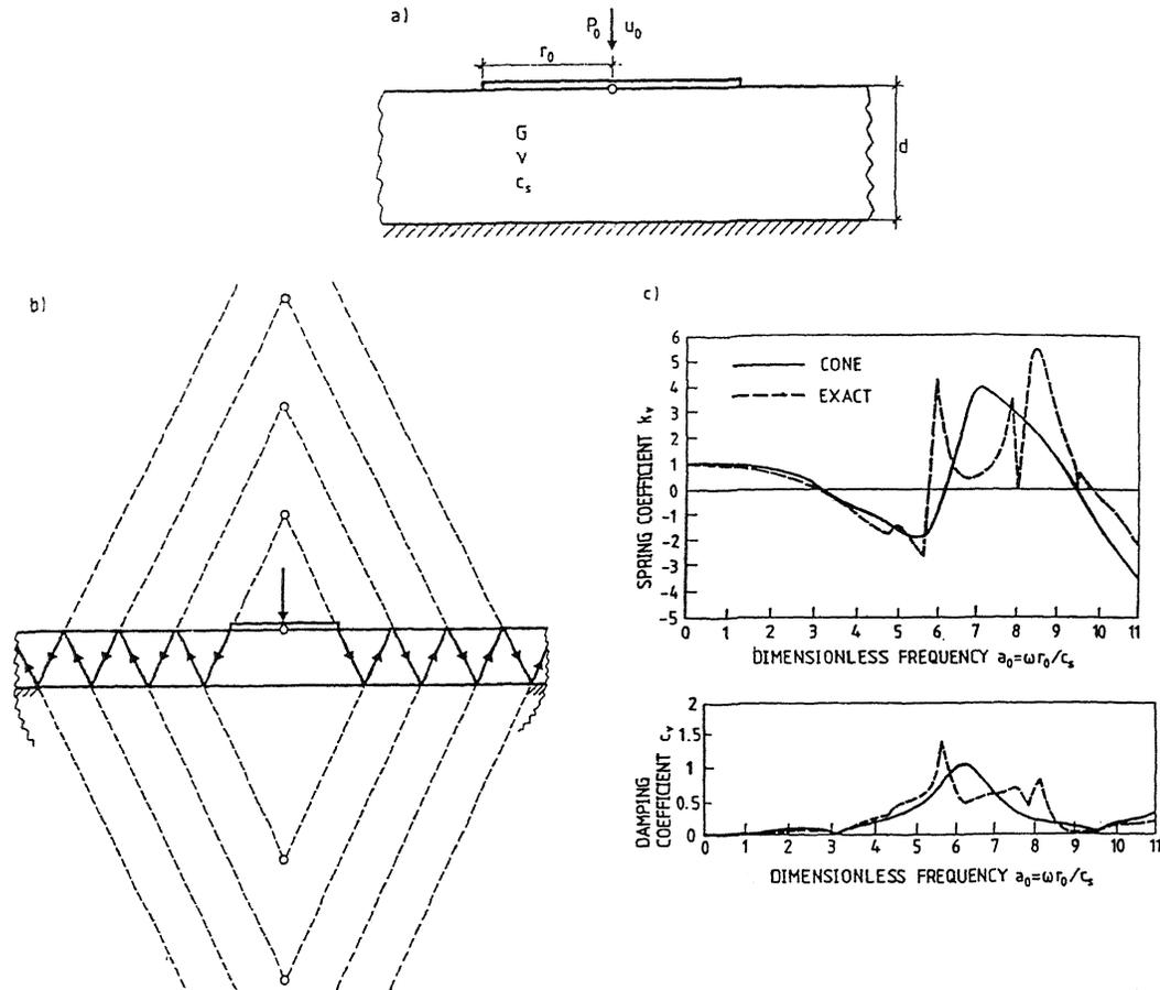
Figure 1. Vertical motion of surface foundation on soil layer on rigid rock.
