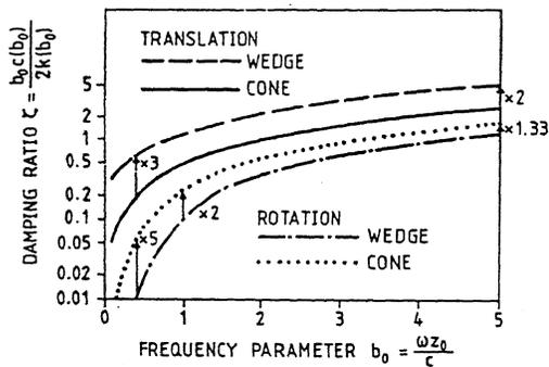
Figure 9. Comparison of three-dimensional modelling (cone) and two-dimensional modelling (wedge).
