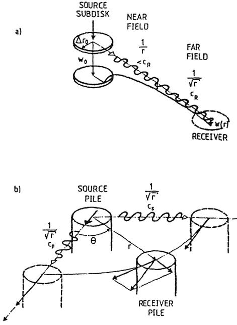
Figure 6. Displacement patterns in horizontal plane.
