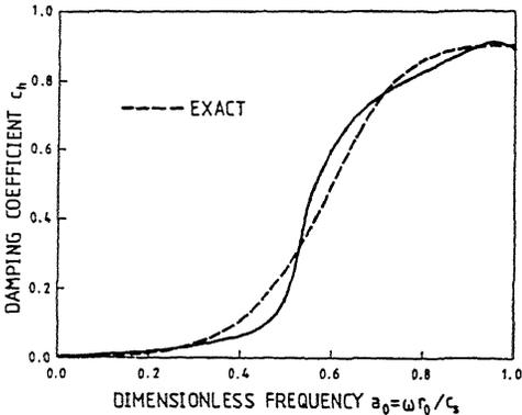
Figure 5. Coupled horizontal and rocking motions of cylinder embedded in soil layer on rigid rock (Fig. 3a).
