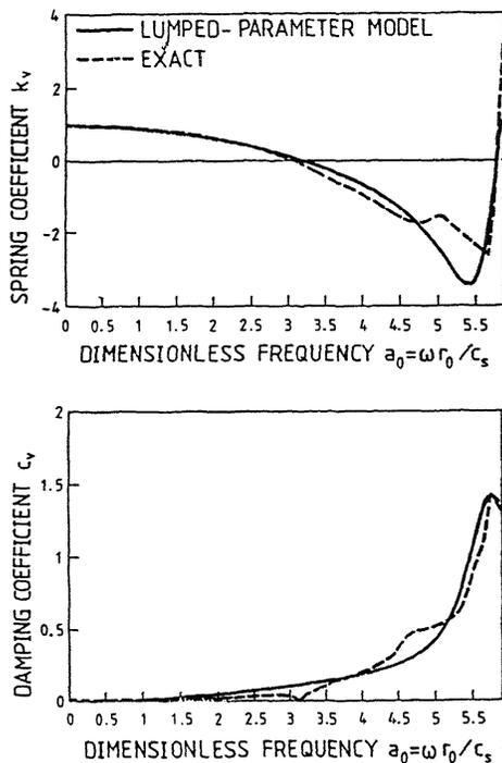
Figure 4. Vertical dynamic-stiffness coefficient of disk on layer on rigid rock (Fig. 1a) calculated with lumped-parameter model of Fig. 2h.
