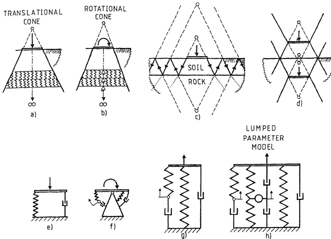
Figure 2. Cones and lumped-parameter models.
