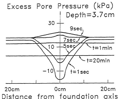
Figure 8. Observed pore pressure isochrones at a depth of 3.7 cm during centrifuge model test of Fig. 6.
