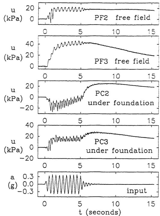
Figure 7. Acceleration and pore pressure records obtained during centrifuge model test of Fig. 6.
