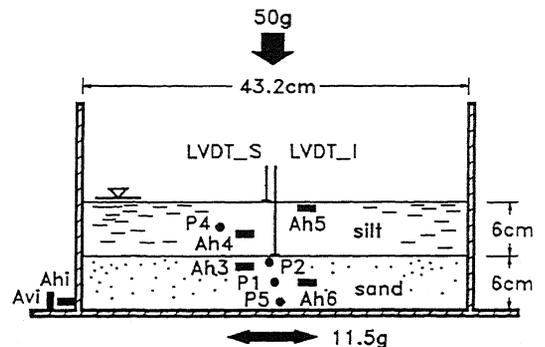
Figure 4. Model of two-layer soil deposit used in centrifuge test
