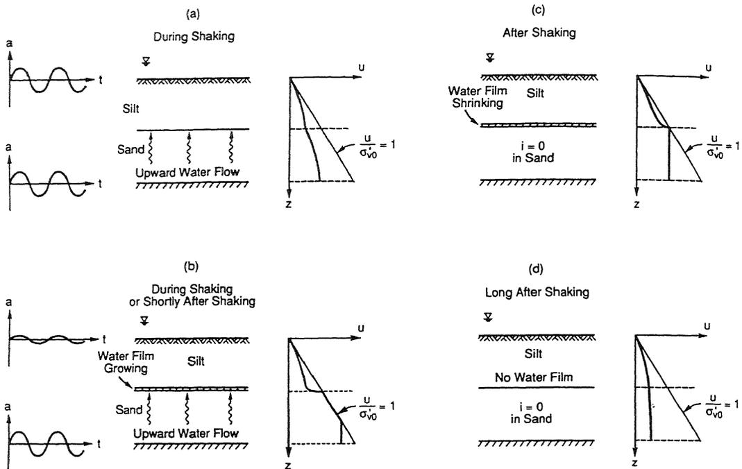
Figure 5. Four stages observed in centrifuge test of two-layer deposit.
