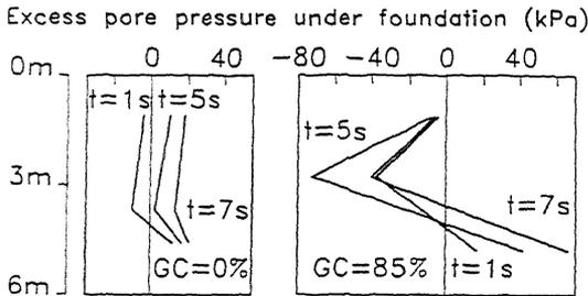
Figure 14. Comparison of pore pressure isochrones under the foundation measured in two tests having different soil permeabilities.
