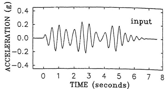
Figure 2. Horizontal acceleration in prototype units measured at base of model during a centrifuge test
