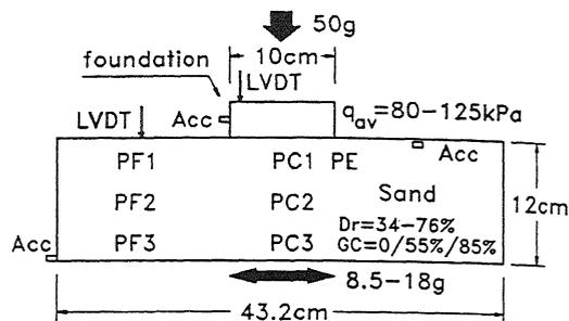
Figure 10. Centrifuge model of shallow foundation on uniform saturated cohesionless deposit.
