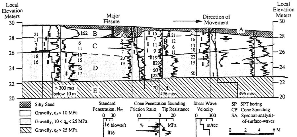
Figure 3. Cross section of liquefaction-induced lateral spread at Pence Ranch site during the 1983 Borah Peak, Idaho earthquake (Andrus, et al., 1991).
