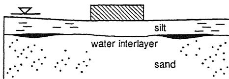
Figure 9. Inferred pattern of water interlayer formation due to shaking of surface foundation on two-layer soil deposit.
