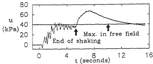
Figure 13. Pore pressure record under the foundation obtained in a uniform sand model with high pore fluid viscosity ( $GC = 85\%$ ).
