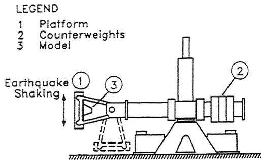
Figure 1. Sketch of RPI geotechnical centrifuge
