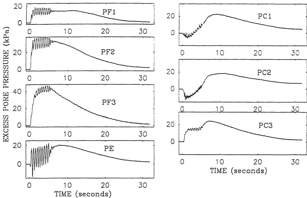
Figure 12. Pore pressure records obtained in centrifuge model test of Figs. 10 and 11.
