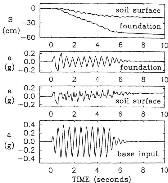
Figure 11. Acceleration and settlement records obtained during one of the centrifuge model tests sketched in Fig. 10.
