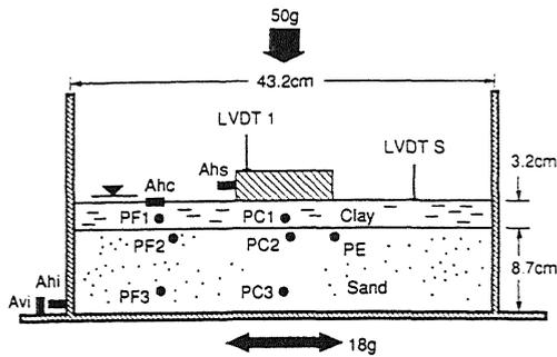
Figure 6. Model of shallow foundation on two-layer soil deposit used in centrifuge test
