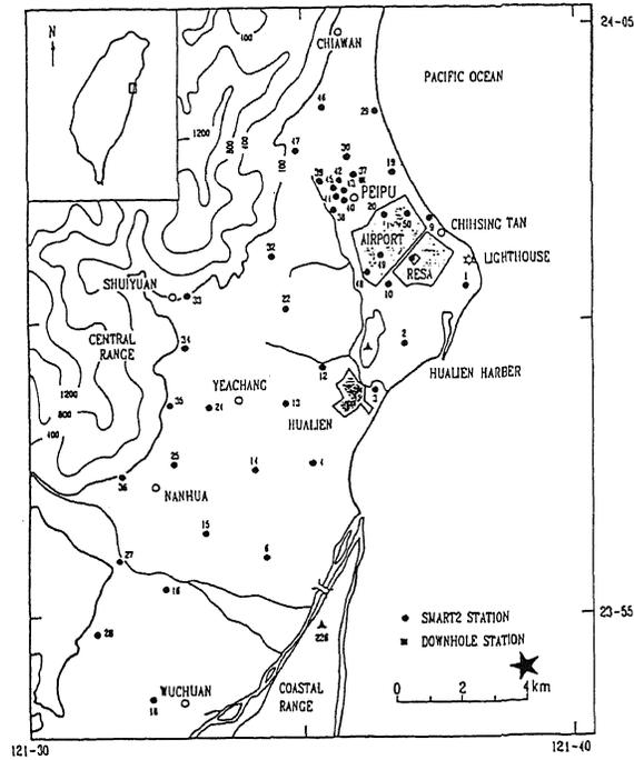
Figure 1. Strong-Motion accelerographs layout for SMART-2 array; solid circle and square represent the free-field and downhole locations respectively. Symbol '★' denotes the epicenter of earthquake December 29, 1990.
