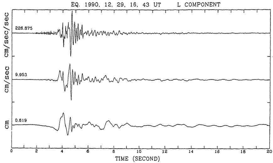
Figure 3. The integrated time histories of velocity and displacement corresponding to the accelerogram recorded by SMART-2 array at S03 (L-component) in December 29, 1990 Hualien earthquake.
