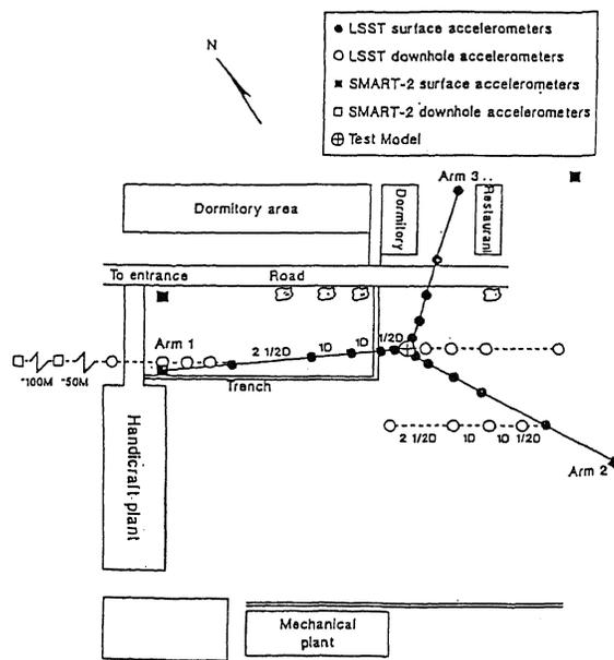
Figure 2. Free-field instrumentation layout for the Hualien LSST project.
