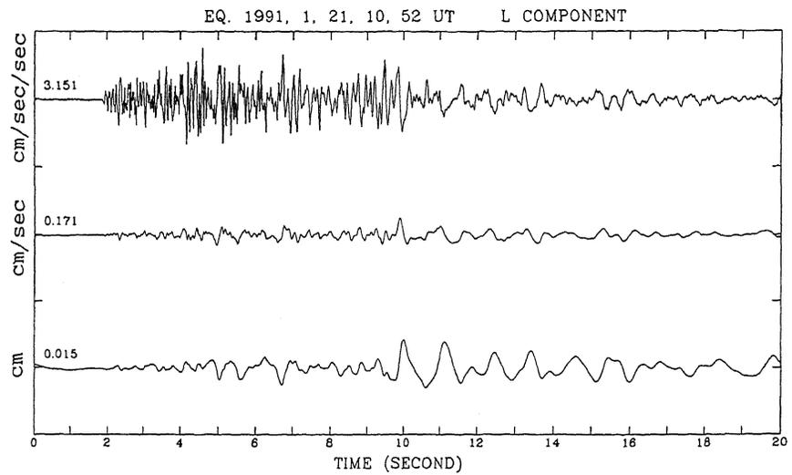
Figure 4. The integrated time histories of velocity and displacement corresponding to the accelerogram recorded by SMART-2 array at S28 (L-component) in January 21, 1991 Hualien earthquake.
