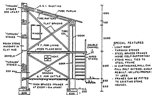
Fig 5. Tubular steel frame with stone wall cladding
