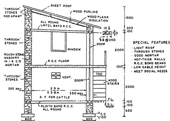
Fig 4. Two storey house with earthquake resistance
