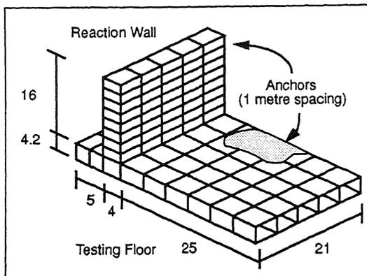
Figure 1: Parameters of the ELSA-Reaction-Wall
