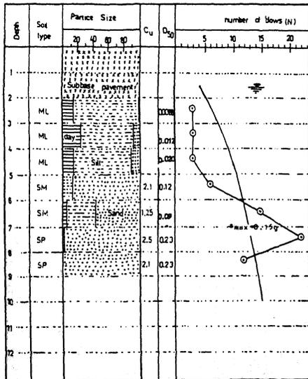
Figure 9. Results of in-situ and laboratory tests on soils present at BH4 (No liquefaction zone).
