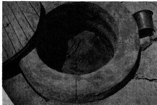
Figure 4. Sand boil from a water well in Astaneh.
