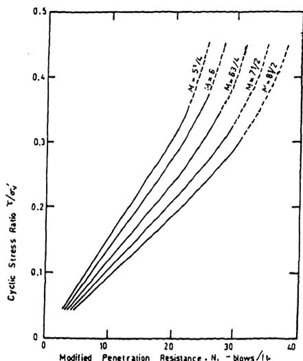
Figure 11. Liquefaction cyclic stress ratio vs modified SPT  $N_1$ -value.
