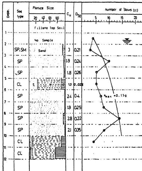
Figure 7. In-situ and laboratory tests on soils present at BH2 (zone of liquefaction).
