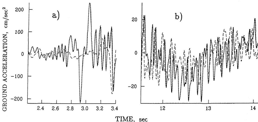
Fig. 6. Actual (solid line), "recorded" (dashed line), and corrected (dotted line) ground acceleration for two time intervals shown in the boxes in Fig. 5.
