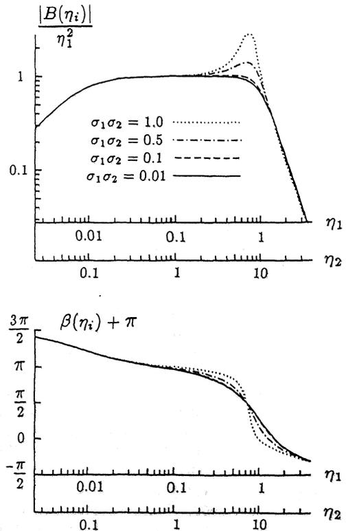
Fig. 1. Sample response of coupled transducer galvanometer system.  $\sigma_2 = 1$ ,  $\xi_1 = 0.6$ ,  $\xi_2 = 6.0$ ,  $\eta_2/\eta_1 = 10$ .
