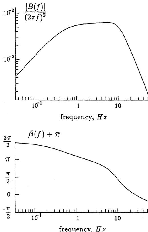
Fig. 4. The amplitude (top) and phase (bottom) transfer function for the device with parameters: transducer natural frequency 5 Hz and ratio of critical damping 5, galvanometer natural frequency 10 Hz and ratio of critical damping 0.6, and coupling constants  $\sigma_1 = 0.01$  and  $\sigma_2 = 1$ .
