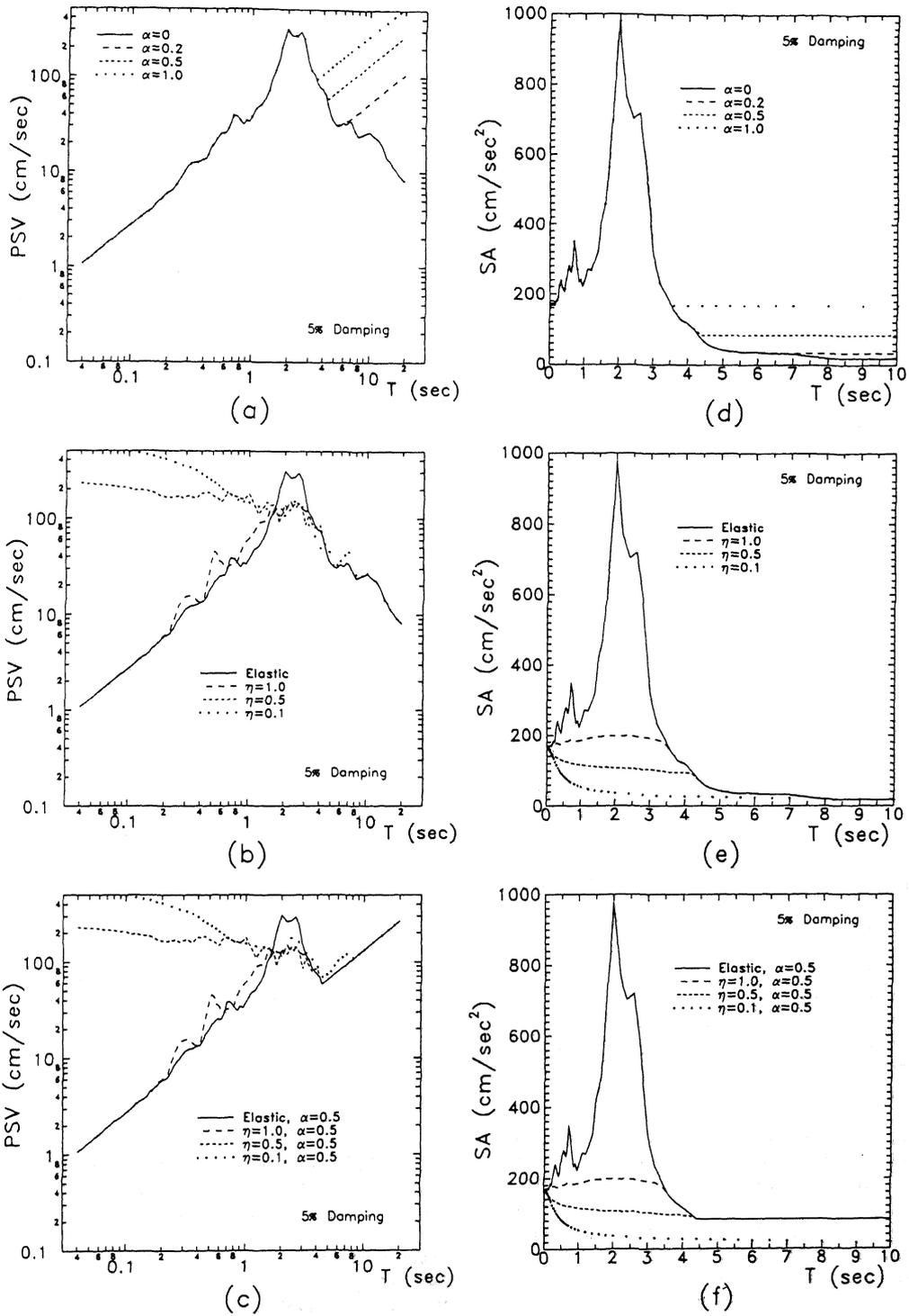
Figure 3. Influence of initial displacement ( $\alpha$ ) on pseudo-velocity (PSV) and absolute acceleration (SA) response spectra for elastic and elasto-plastic systems subjected to Mexico 1985 earthquake.
