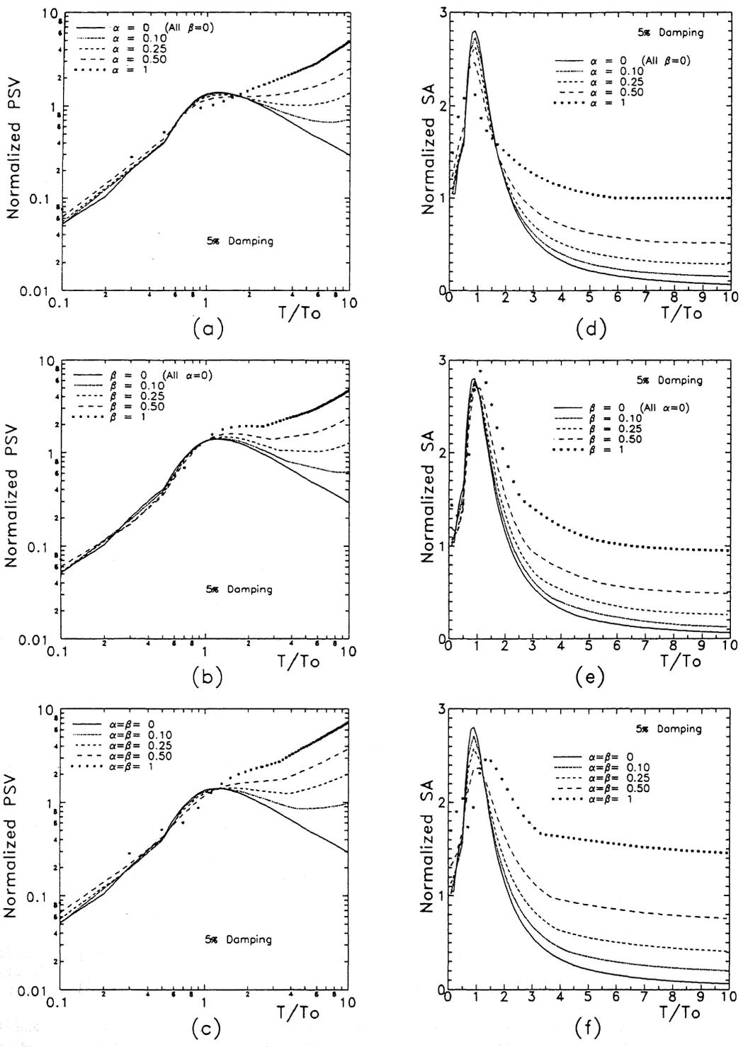
Figure 1. Influence of initial displacement ( $\alpha$ ) and initial velocity ( $\beta$ ) on pseudo-velocity (PSV) and absolute acceleration (SA) response spectra for elastic systems subjected to sinusoidal base excitation.
