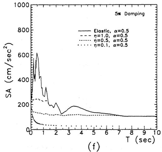
Figure 2. Influence of initial displacement ( $\alpha$ ) on pseudo-velocity (PSV) and absolute acceleration (SA) response spectra for elastic and elasto-plastic systems subjected to El Centro 1940 earthquake.
