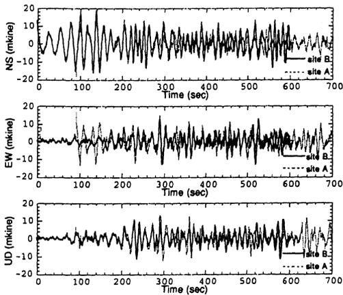
Figure 5. Velocity time histories of No. 17 Myanmar earthquake.
