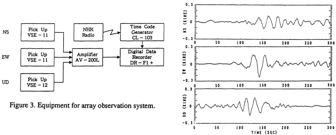
Figure 3. Equipment for array observation system.
