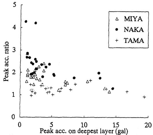
Figure 7 Vertical peak acceleration ratios on surface to deepest layer
