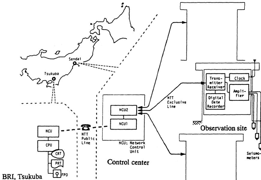
Figure 3 Block diagram of observation system
