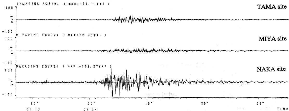
Figure 5 Accelerograms on the ground surface for the earthquake #8724 (NS component)
