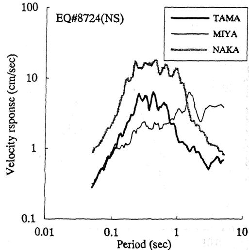
Figure 8 Response spectra on surface for eq. #8724
