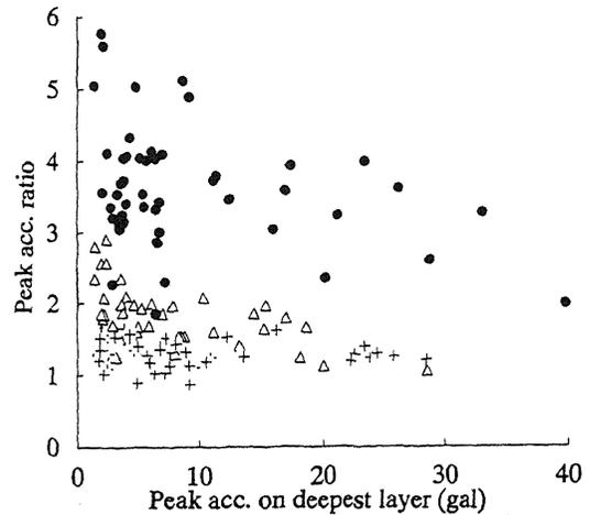
Figure 6 Horizontal peak acceleration ratios on surface to deepest layer
