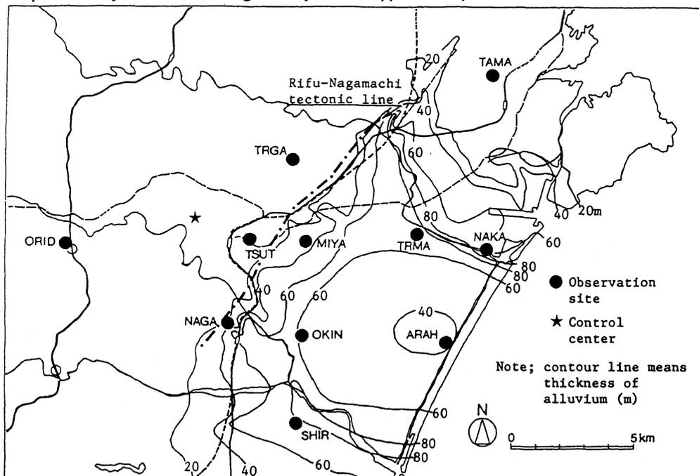
Figure 1 Layout of observation sites and a control station, and thickness of alluvium
