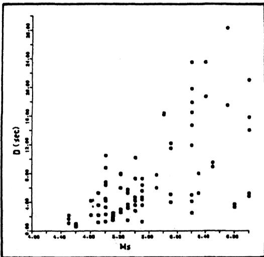
Fig.1 Distribution of S.M.D.,  $D$ , versus surface wave magnitude,  $M_s$ .
