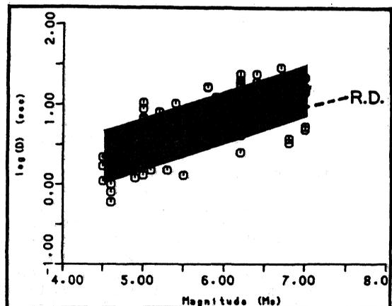
Fig.3 Comparison of S.M.D.,  $D$ , and rupture duration,  $R.D.$ , versus surface wave magnitude,  $M_s$ .
