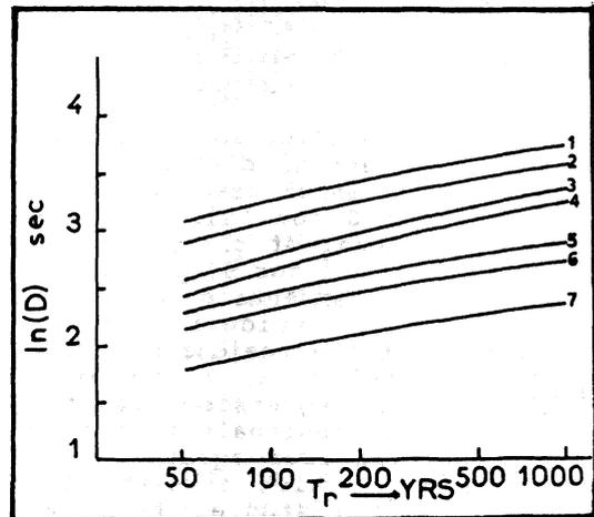
Fig.7. Seismic hazard curves of S.M.D. versus the mean return period,  $T_r$ , for the 7 examined sites in Greece.
