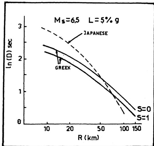
Fig.5. Comparison between the Greek, for two soil conditions (solid lines) and Japanese (dashed line) S.M.D. reduced to  $M_s=6.5$ , and  $L=5\%g$ .
