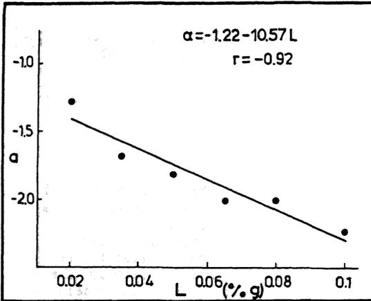
Fig.4 Coefficient  $a$ , versus threshold level of acceleration,  $L$ .
