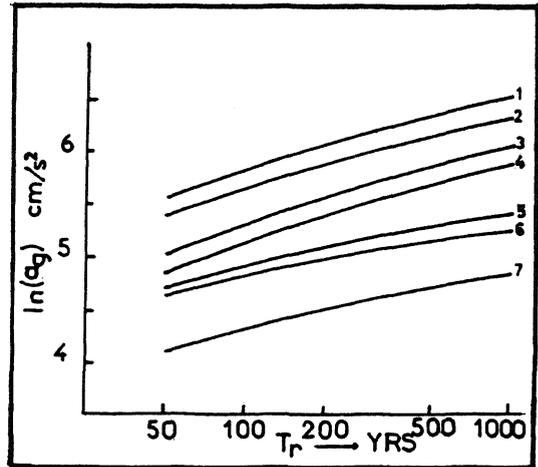
Fig.6. Seismic hazard curves of P.G. acceleration versus the mean return period,  $T_r$ , for the 7 examined sites in Greece.
