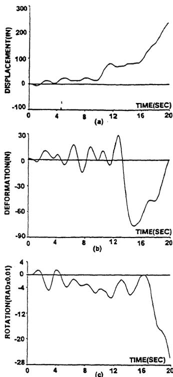
Figure 11. Responses at top floor's mass center (a) in X direction, (b) in Y direction, and (c) in Z direction
