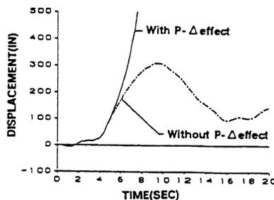
Figure 10. Comparison of structural responses at top floor mass center
