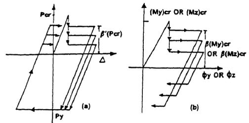
Figure 8. Hysteresis model for local-buckling columns, (a) axial load, (b) bending moment
