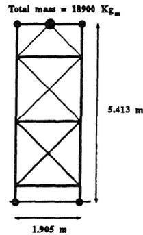
Figure 1: Jacket-type offshore platform 2D frame
