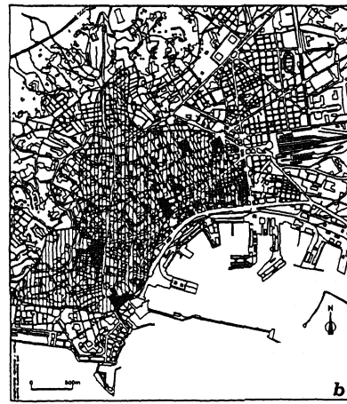
Fig.4 (a) The 5th June, 1688 Campania earthquake. The intensity in Naples reached the VII-VIII MCS (Serva, 1985). (b) Damages scenario in Naples: the hatched area shows the type of damage suffered by the historical Centre, black colored buildings are the monumental buildings reported into the historical documents. Statistics: 3% great damage with partial collapse; 5% serious damage, deep damage; 91 % slight damage, little damage.
