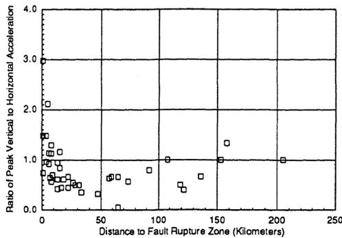
Fig. 2 Ratio of Vertical to Average of Horizontal Peak Ground Accelerations for the Imperial Valley Earthquake.
