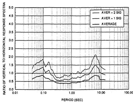
Fig. 11 Ratio of Vertical to Horizontal Response Spectra for 5% Damping - Loma Prieta Earthquake
