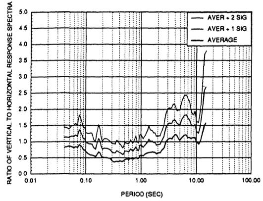
Fig. 6 Ratio of Vertical to Horizontal Response Spectra for 5% Damping - Coalinga Event 2
