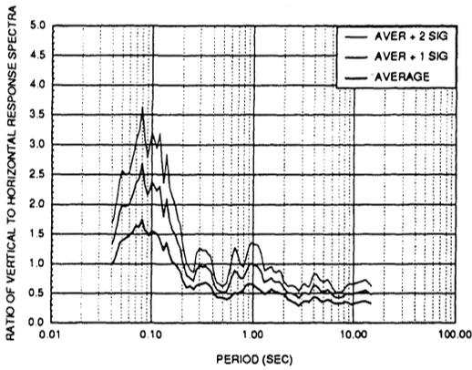
Fig. 4 Ratio of Vertical to Horizontal Response Spectra for 5% Damping - Imperial Valley Earthquake
