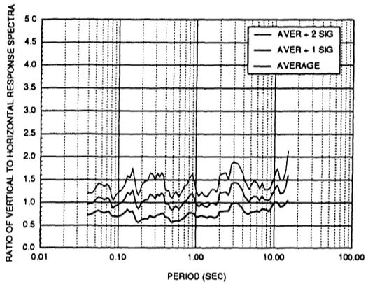
Fig. 7 Ratio of Vertical to Horizontal Response Spectra for 5% Damping - Coalinga Events 3 to 9
