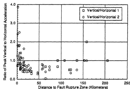
Fig. 1 Ratio of Vertical to Horizontal Peak Ground Accelerations for the Imperial Valley Earthquake.
