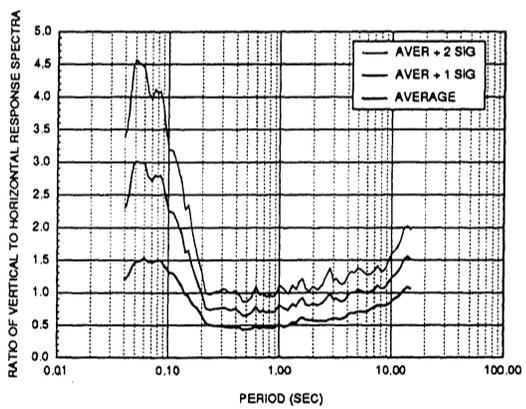
Fig. 8 Ratio of Vertical to Horizontal Response Spectra for 5% Damping - Morgan Hill Earthquake
