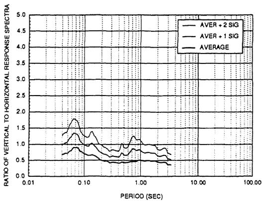
Fig. 10 Ratio of Vertical to Horizontal Response Spectra for 5% Damping - Whittier Narrows Earthquake
