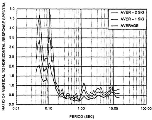
Fig. 5 Ratio of Vertical to Horizontal Response Spectra for 5% Damping - Westmorland Earthquake
