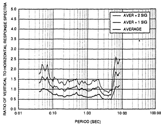
Fig. 9 Ratio of Vertical to Horizontal Response Spectra for 5% Damping - Palm Springs Earthquake
