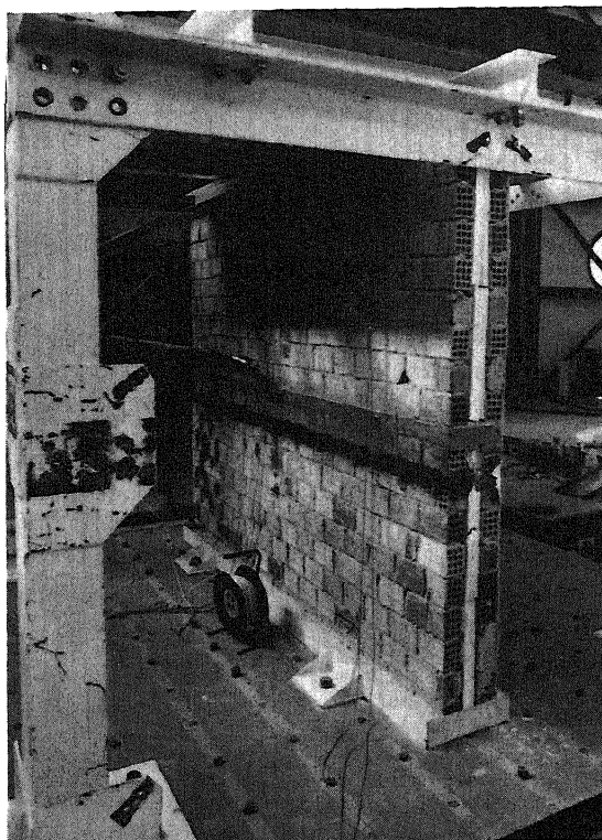
Fig.18. View of the test set-up after the excitation with twenty repetitions of the desctrutive Kalamata earthquake.
