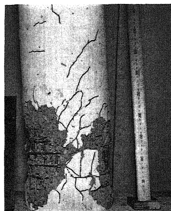
Figure 11. Hinge region of Pier 11 at collapse
