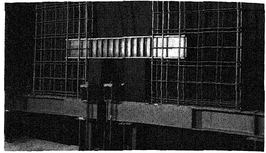
Figure 1. Overall view of reinforcing cage and coupling beam of Specimen 1.
