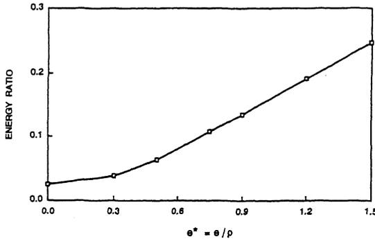
Figure 7. Energy dissipated by yielding in friction damped frames with respect to unbraced frames.
