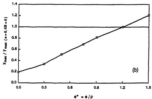
Figure 5. Displacement of optimized friction damped structures normalized with respect to corresponding: (a) unbraced eccentric structure; (b) unbraced symmetric structure.
