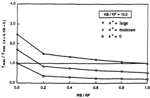
Figure 3. Effect of bracing stiffness KB and slip load RB on eccentric response.
