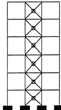
(b) Typical Frame with Friction Damped Bracing
