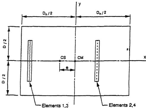
Figure 2. One-story model of friction damped asymmetric structure.
