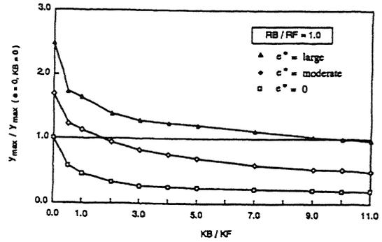
Figure 4. Effect of bracing stiffness KB at optimum slip load.
