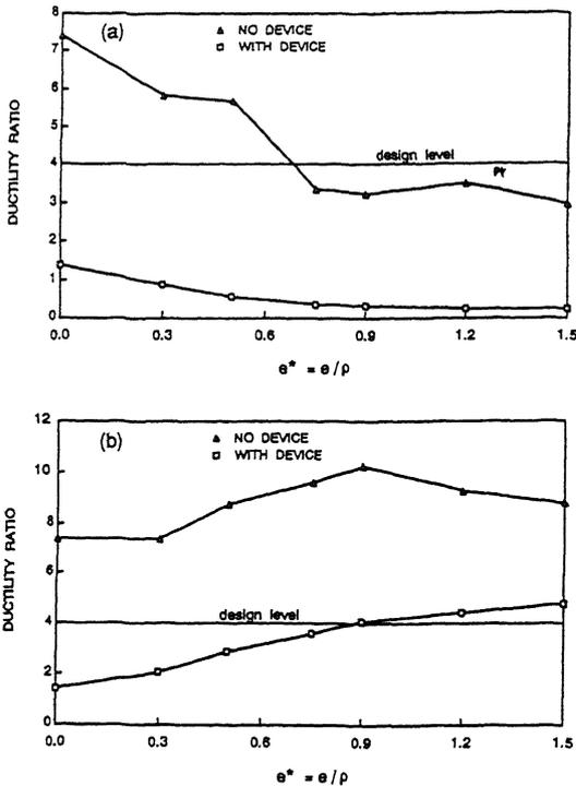
Figure 6. Effect of friction devices on ductility demand for frames on: (a) stiff side; (b) flexible side.
