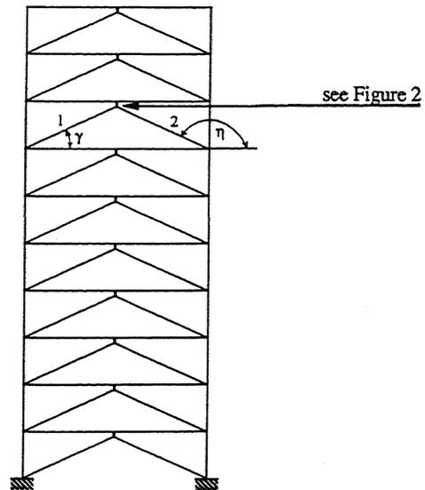
Figure 1. Typical ADAS installation in a building frame.
