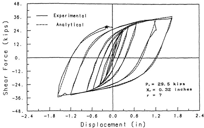
Figure 5. Hysteresis correlation between experimental and analytical results for the bottom device of the concrete frame. (1 in. = 25.4 mm, 1 kip = 0.225 kN)
