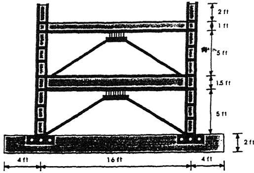
Figure 3. Concrete frame strengthened with ADAS devices. (1 ft = 12 inches = 305 mm = 0.305 m)
