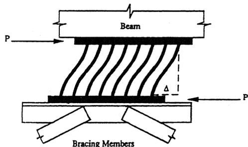
Figure 2. ADAS device in its deformed condition.
