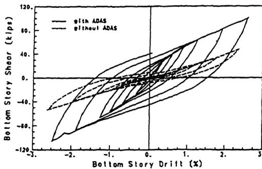
Figure 4. Hysteresis curves for bottom story of the reinforced concrete frame before and after installation of ADAS devices. (1 kN = 4.45 kips)
