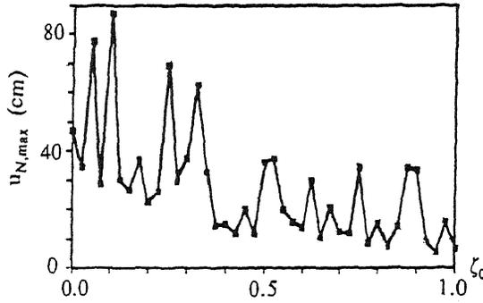
Figure 4. The influence of damping ratio on maximum top floor displacement
