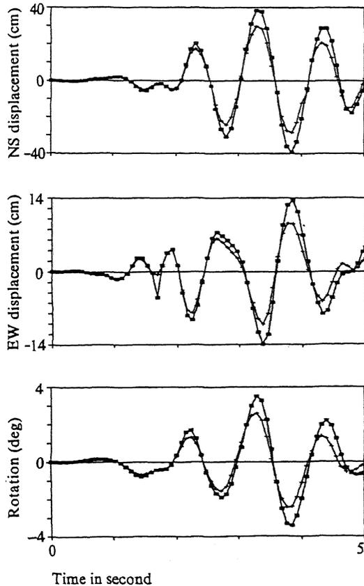
Figure 5. Coupled lateral and torsional seismic responses of a 3-D building with or without optimal damper control
