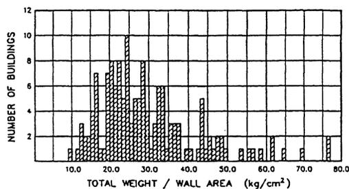
Figure 3. Number of buildings as a function of shear index.
