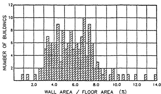
Figure 2. Number of buildings as a function of the amount of cross sectional area of walls.
