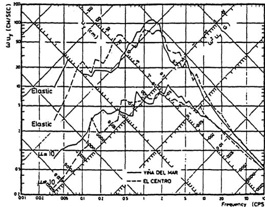
Figure 1. Comparison of spectra for Viña del Mar and El Centro, 5% damping, elastic and inelastic for ductility factor of 10.
