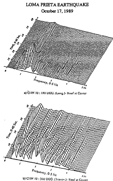
Figure 1. Time dependent spectra from two different records
