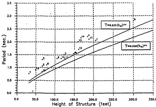
Figure 3. Period versus height for RC/MRF
