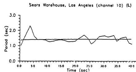
Figure 2. Time variation of building period with logarithmic fit.
