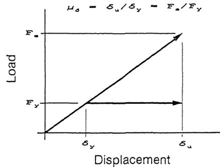
Figure 6 - Displacement Ductility Based on Equal Displacement Rule
