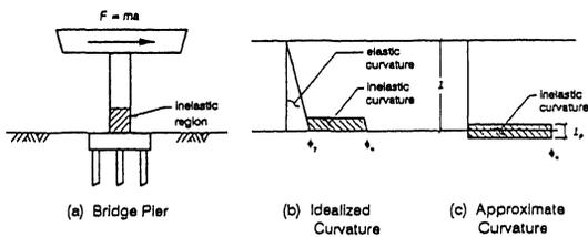
Figure 3 - Simplified Curvature Distribution in Cantilever Bridge Pier
