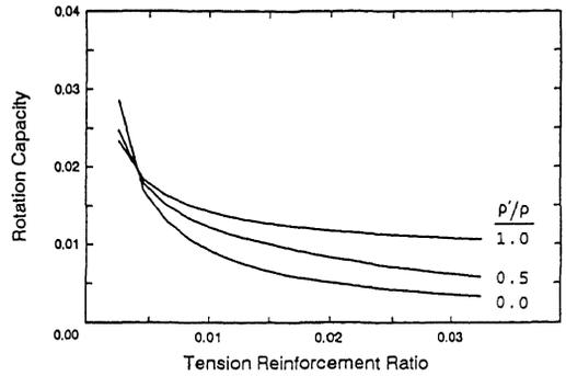
Figure 5 - Rotational Capacity of Reinforced Concrete Beam Sections
