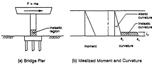
Figure 2 - Idealized Flexural Curvature in Cantilever Bridge Pier
