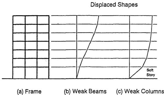
Figure 1 - Building Frame Deformation Modes
