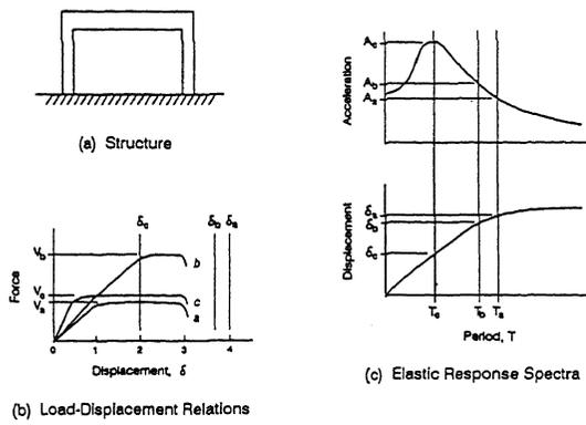
Figure 7 - Example Redesign of Existing Frame
