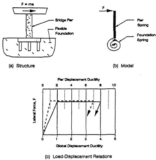
Figure 8 - Bridge Pier with Flexible Foundation
