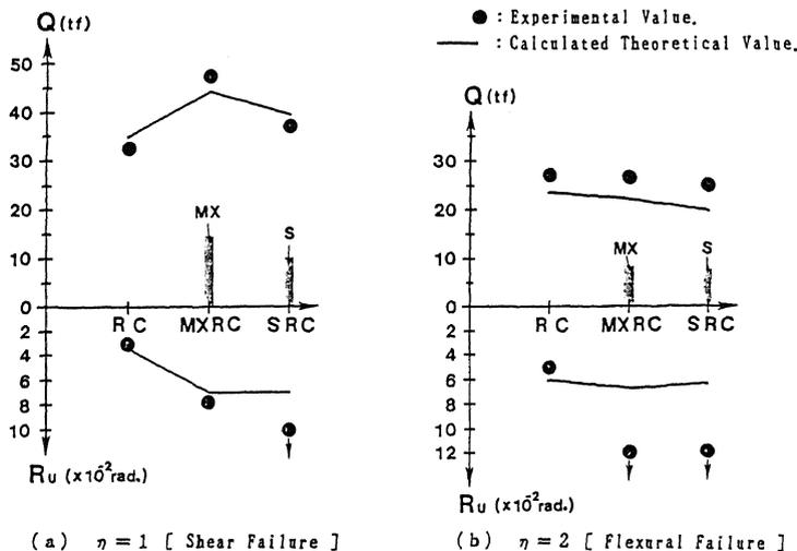
Fig. 5. Correlation between Ultimate Strength ( $Q$ ) and Critical Joint Translation Angle ( $R_{UJ}$ ), and RC, MXRC, SPC
