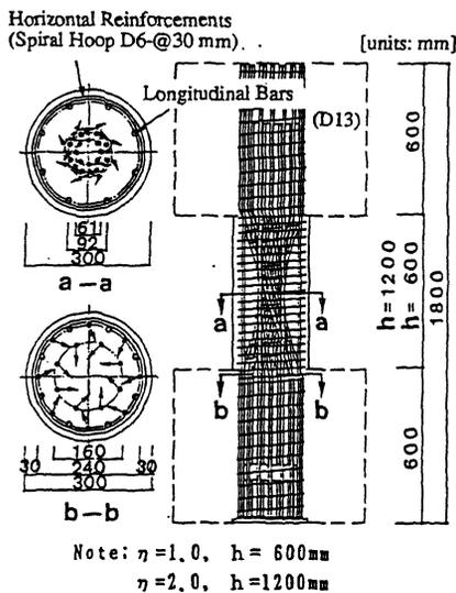
Fig. 3. Test Specimens of MXRC
