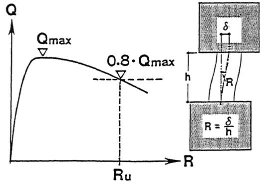
Fig. 6. Definition of the Critical Joint Translation angle,  $R_U$
