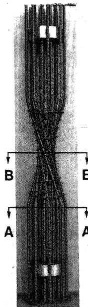
Photo 1. Arrangement of MX Reinforcement System
