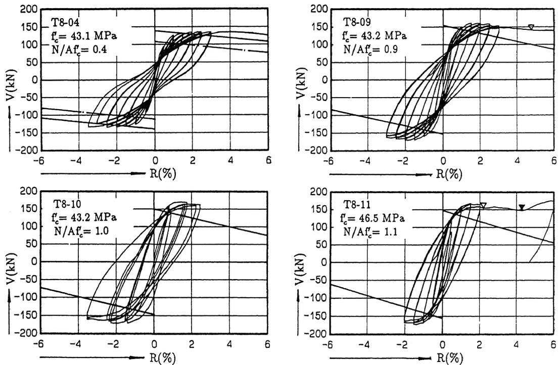
Figure 4 Lateral load  $V$  - translation angle  $R$  relationships for wholly confined specimens
