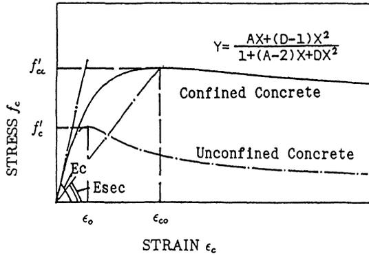
Figure 5 Proposed stress-strain curve for concrete
