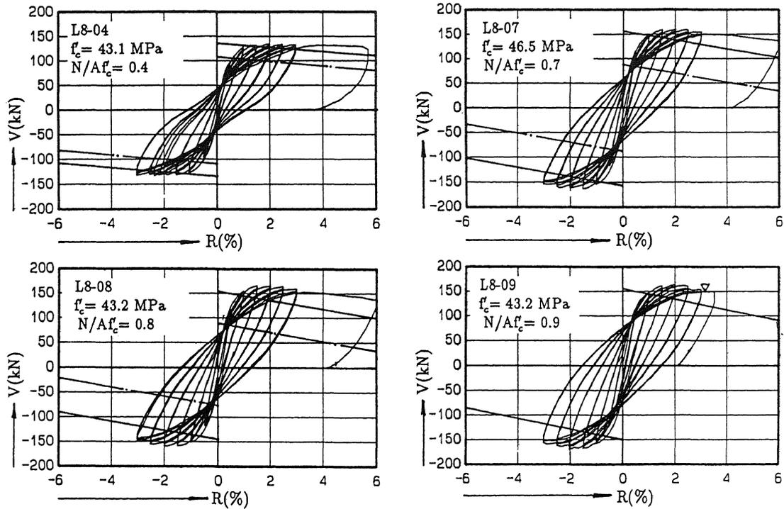
Figure 3 Lateral load  $V$  - translation angle  $R$  relationships for locally confined specimens
