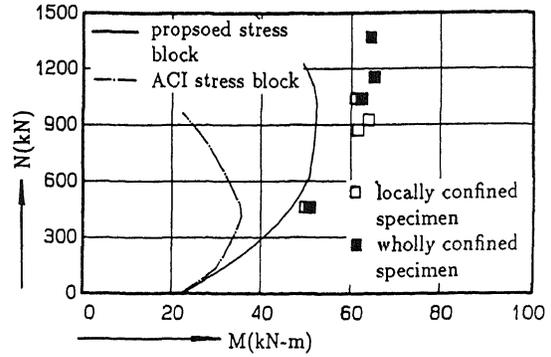
Figure 6 Comparison between the experimental and theoretical ultimate moment
