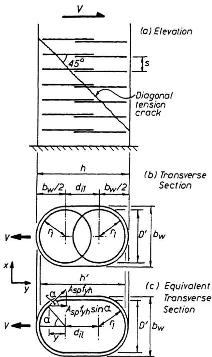
Fig.2 Shear carried by interlocking spirals.
