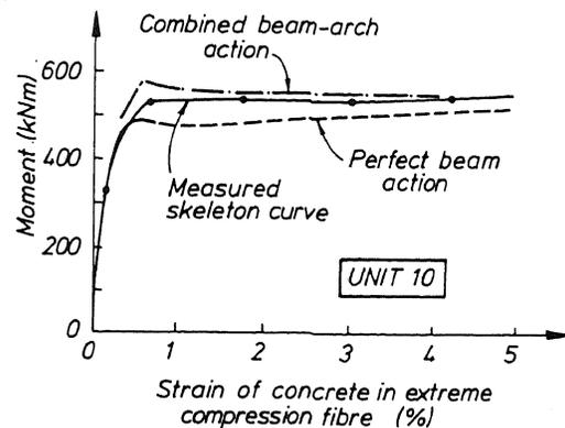
Fig.10 Comparison between theoretical and measured moment-concrete strain relations for Unit 10.
