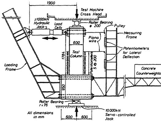
Fig. 6 Loading arrangements for Units 9 to 12.
