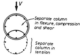
Fig.9 Assumed separate columns for combined beam-arch action models.
