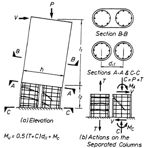
Fig.3 Combined beam-arch action model for the case when the interlock of spiral is weak.
