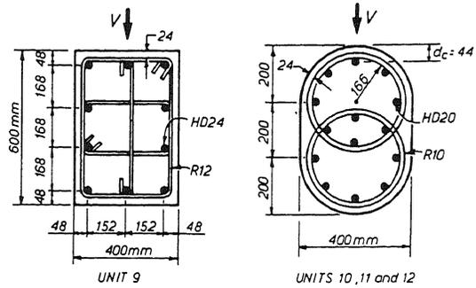
Fig.5 Column section details for Units 9 to 12.
