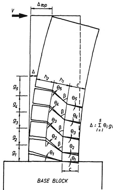
Fig.11 Assumed shear deformation model.
