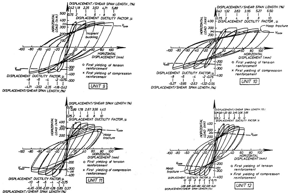
Fig.7 Measured horizontal load-horizontal displacement hysteresis loops for Units 9 to 12
