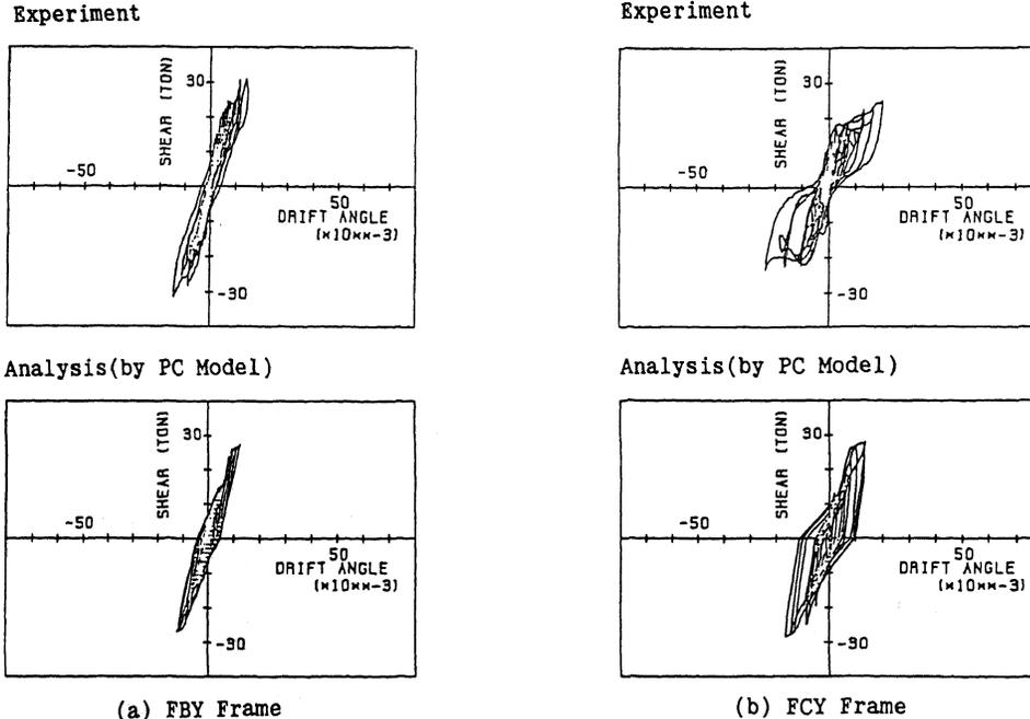
Figure 9. Comparison of base shear force versus roof drift angle relationships between experiments and analyses
