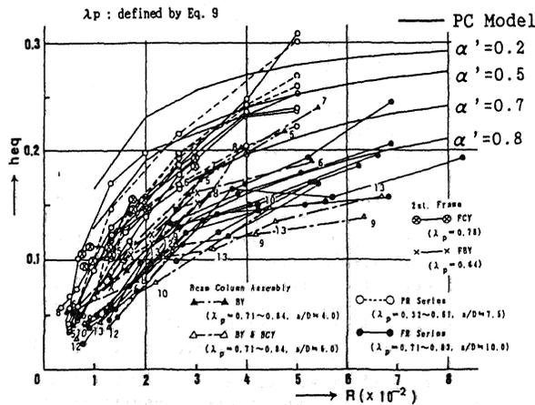
Figure 2. Equivalent viscous damping factor versus drift angle relationship
