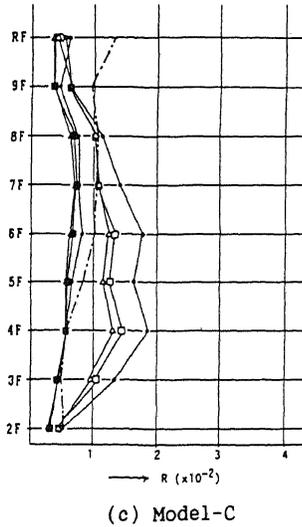
Figure 3. Results of nonlinear dynamic analyses on multi story PC buildings using PC Model
