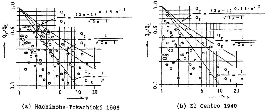
Figure 5. Response ductility factor( $\alpha'=0.8$ )
