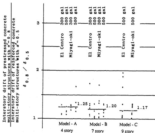
Figure 4. Increased response of PC multi degree-of-freedom system
