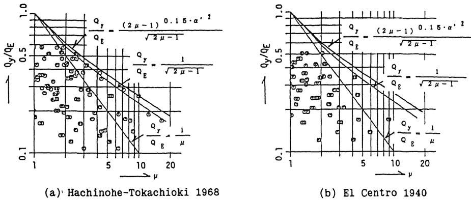
Figure 6. Response ductility factor( $\alpha'=0.5$ )
