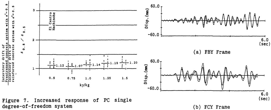
Figure 7. Increased response of PC single degree-of-freedom system
