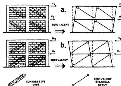
Figure 6. Configurations with the diagonal strut analogy.
