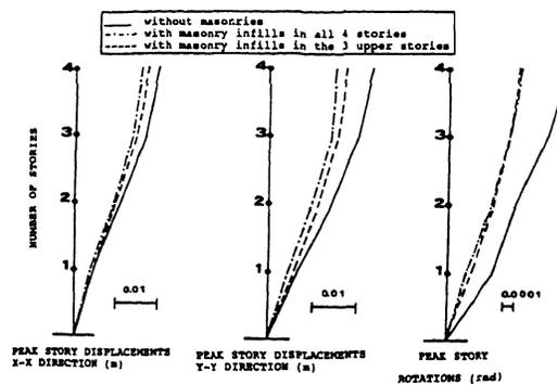
Figure 8. Peak story displacements from the dynamic elastic analyses.
