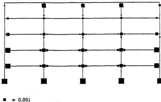
Figure 4. Damage index for the SMRSF frame subjected to accelerogram no. 49 for the Imperial Valley site.
