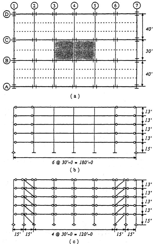
Figure 1 (a) Plan view of building. (b) Elevation of SMRSF and OMRSF. (c) Elevation view of CBF.
