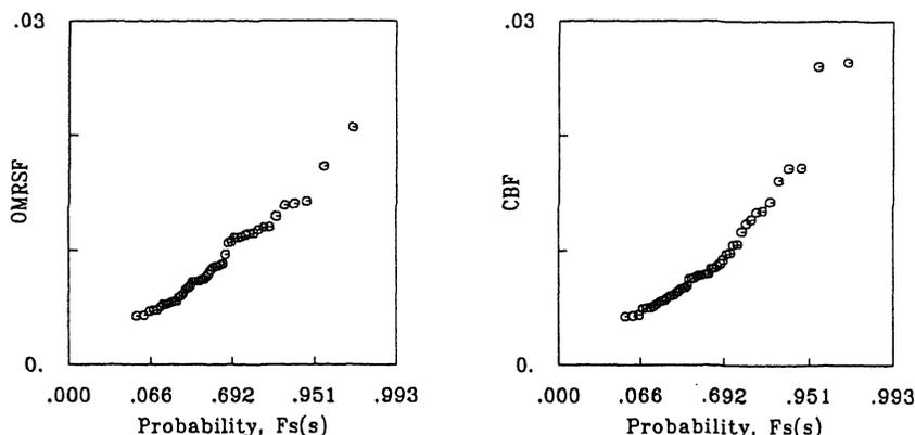
Figure 5. Maximum first-story drift plotted on type 1 extreme value probability paper for 50 Imperial Valley accelerograms for OMRSF and CBF frames.
