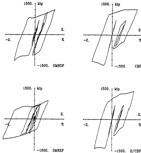
Figure 3. Strong shear vs. drift for the first story of each building subjected to accelerogram no. 49 for the Imperial Valley site.
