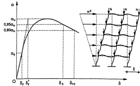
Figure 1. Multiplier of horizontal forces versus top displacement curve
