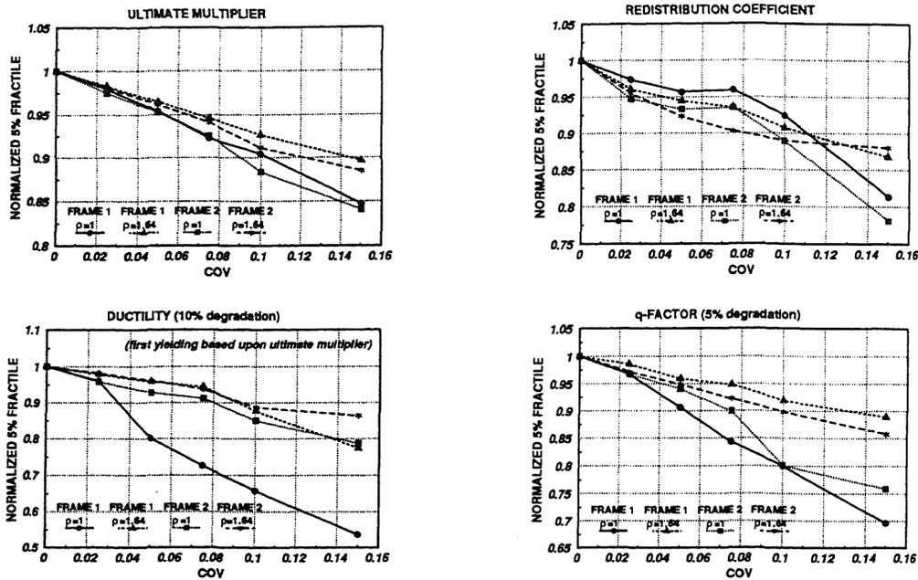
Figure 4. Influence of the column-to-beam strength ratio and of the structural scheme.
