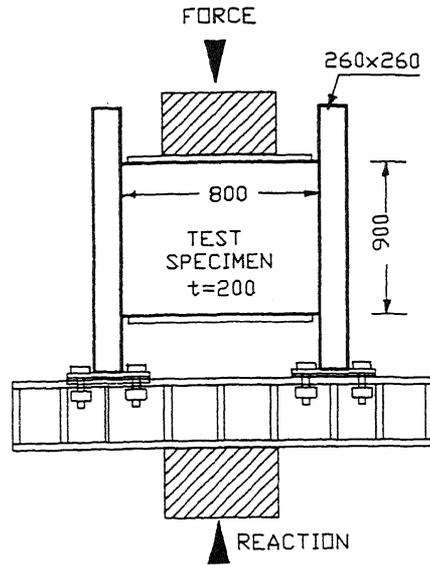
Figure 7. Test setup
