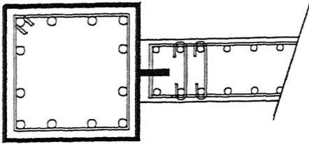
Figure 6. Interface connection with perfobond strips
