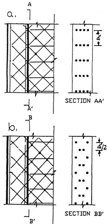
Figure 4. Interface connection with diagonal reinforcing bars
