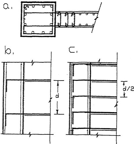
Figure 3. Interface connection with horizontal reinforcing bars
