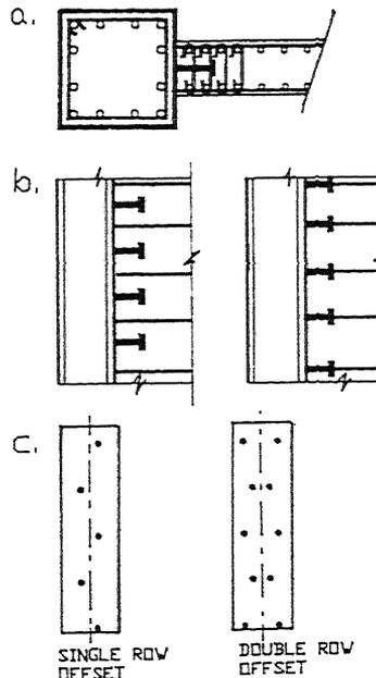
Figure 5. Interface connection with headed studs (19mm dia.)
