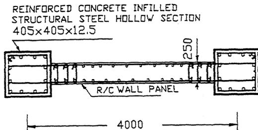
Figure 2. Composite structural wall
