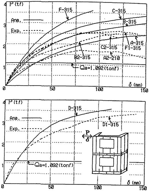
Figure 3. Skeleton curve (test and analysis)
