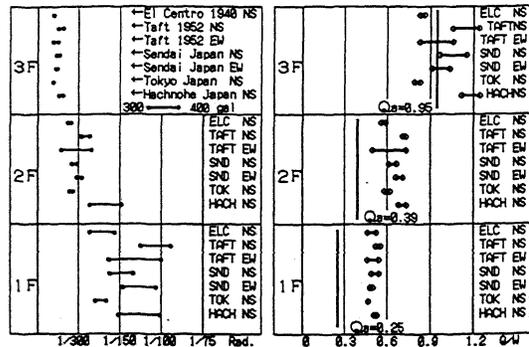
Figure 13. Displacement responses at roofs for recorded seismic waves (300 and 400 gal)
