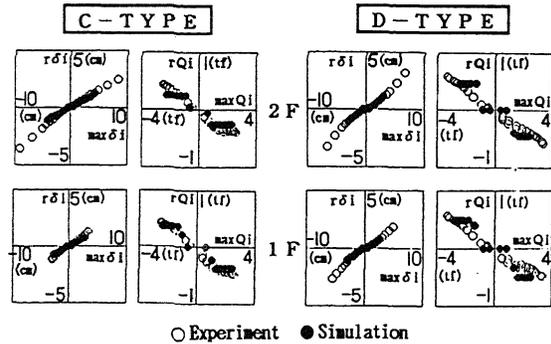
Figure 5. Residual displacements and residual shear force ( : Experiments : Simulations)
