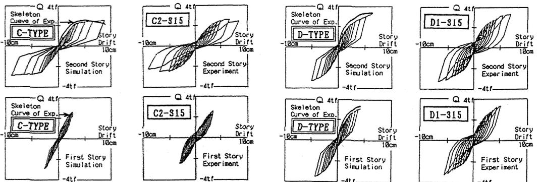
Figure 6. Simulations of hysteresis (compared with the static loading tests)
