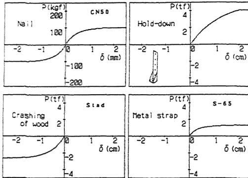
Figure 2. Models of joints for analysis
