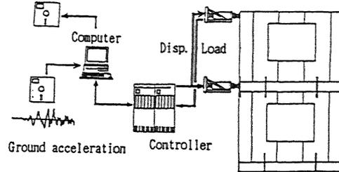
Figure 7. Set-up of pseudo-dynamic tests
