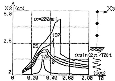
Figure 11. Response spectrum for simple harmonic ground motions (duration time of 8 sec.)
