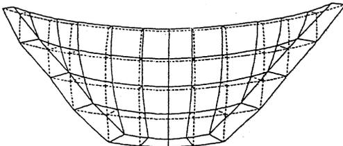
Figure 1 Double curvature arch dam discretized using 3D 20 node and 15 node solid elements.
