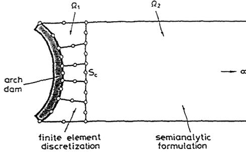
Figure 2 Fluid domain discretization.
