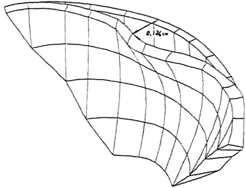
Figure 6 Llauset dam. Deformed shape under response spectrum of Figure 3.
