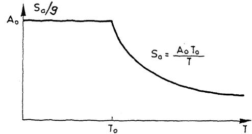
Figure 3 Seismic spectrum considered.
