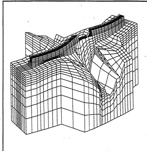
Fig. 3 Cleveland Dam - Fundamental mode shape
