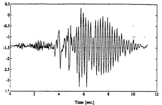
Fig.13 Ambiesta dam: non-linear analysis, displacement Z, node 74 [ $10^{-3}$  m]
