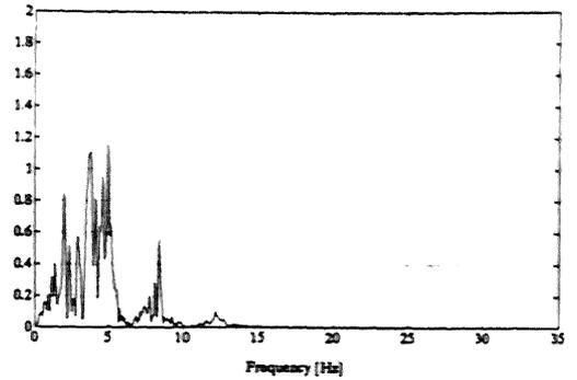
Fig. 17 Ambiesta dam: non-linear analysis, F.T. module of displacement Y node 74, [ $10^{-3}$  m sec]
