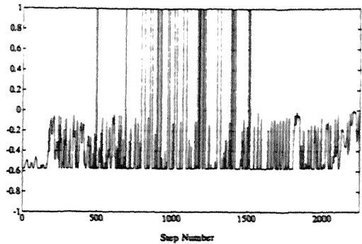
Fig.7 Ambiesta dam: rate between shear stress and normal stress plotted in Figure 6; value 1 means open joint, value -0.578 means plastic sliding.
