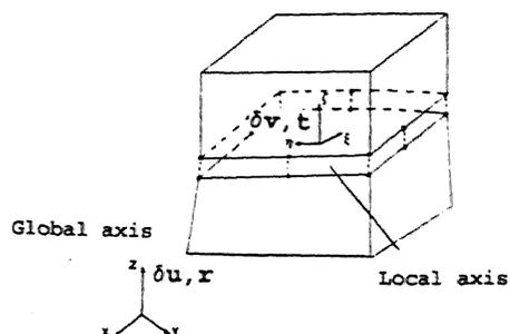
Fig.1 Joint element: geometry, relative displacements field, contact forces
