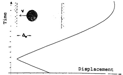
Fig.2 Impact problem: mass-spring model and solution
