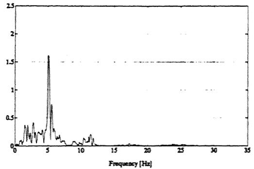
Fig. 18 Ambiesta dam: linear analysis, F.T. module of displacement Z node 74, [ $10^{-3}$  m sec]
