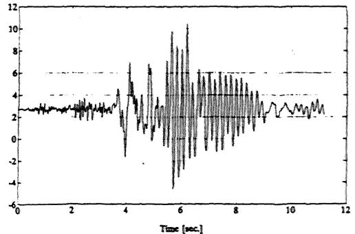
Fig.8 Ambiesta dam: linear analysis, displacement X node 74, [ $10^{-3}$  m]
