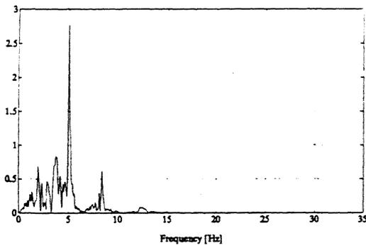
Fig. 16 Ambiesta dam: linear analysis, F.T. module of displacement Y node 74, [ $10^{-3}$  m sec]
