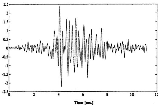
Fig.11 Ambiesta dam: non-linear analysis, displacement Y node 74 [ $10^{-3}$  m]
