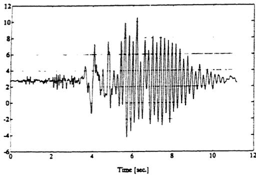
Fig.9 Ambiesta dam: non-linear analysis, displacement X node 74, [ $10^{-3}$  m]
