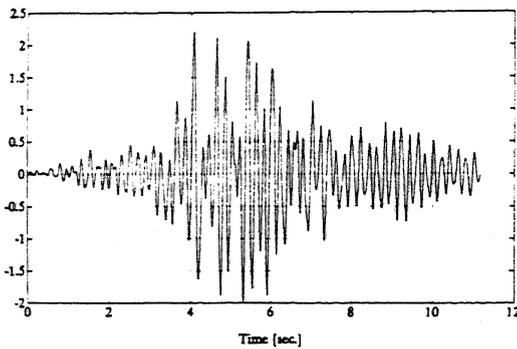
Fig.10 Ambiesta dam: linear analysis, displacement Y node 74, [ $10^{-3}$  m]
