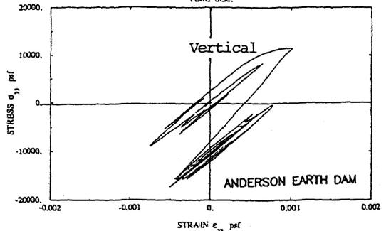
Figures 16, 17. Computed vertical normal stress and strain (with the hysteresis loop) near the crest level of Anderson Dam.
