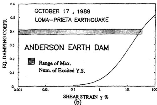
Figures 14, 15. Range of earthquake-induced dynamic shear strain: (a) with shear modulus, and (b) with hysteretic damping coefficient.
