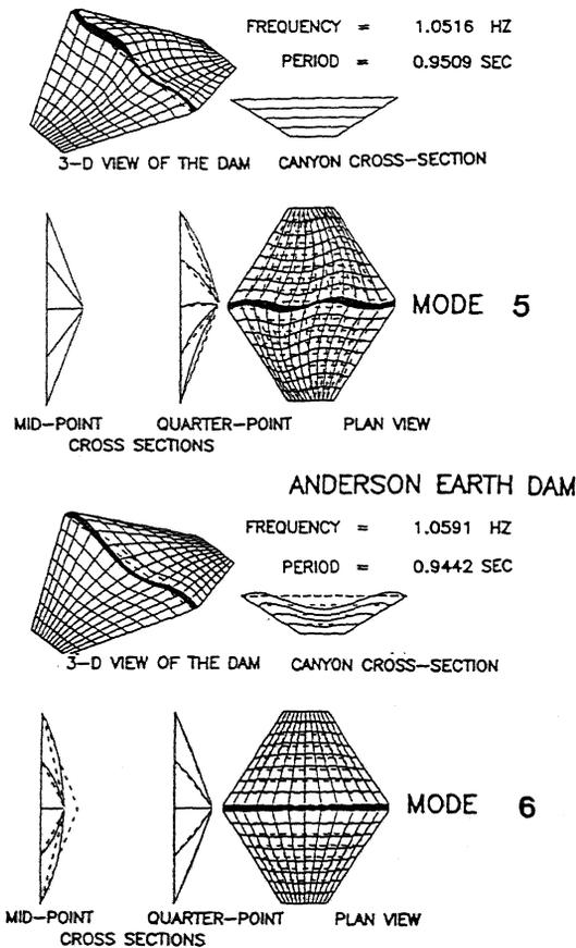
Figure 6. Samples of the global (mode) shape functions.
