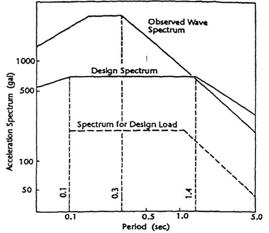
Figure 3. Response Spectra of Input Wave
