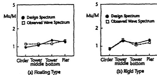
Figure 5. Safety Level by Bending Moment
