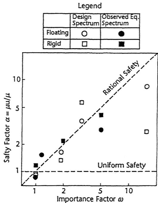
Figure 9. Comparison of Safety Factor with Importance Factor
