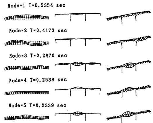
Figure 6. Natural Periods and mode shapes by C M M (rigid connection)
