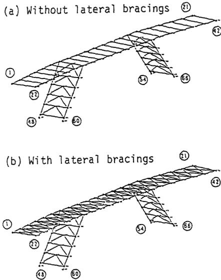
Figure 4. Three-dimensional framework models
