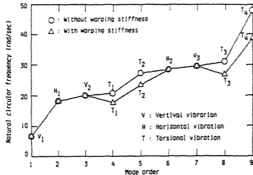
Figure 10. Effect of warping stiffness
