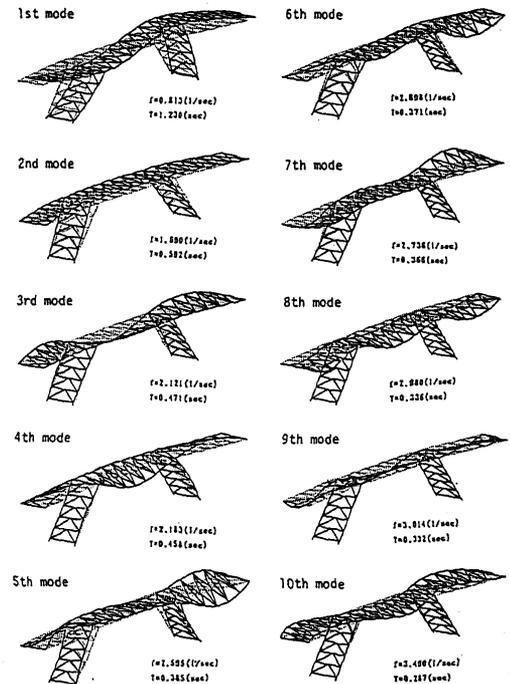
Figure 6. Computed natural mode shapes (with lateral bracing members)
