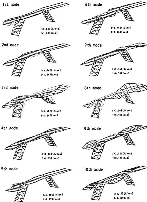
Figure 5. Computed natural mode shapes (without lateral bracing members)
