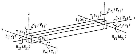
Figure 2. Beam segment of a space frame showing forces and displacements
