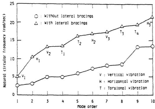
Figure 7. Effect of lateral bracing members
