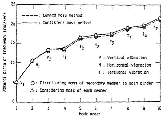
Figure 8. Effect of mass of structural beam members
