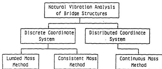
Figure 1. Schematic description of coordinate systems
