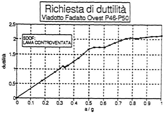
Fig. 8 Ductility demand for the design without dissipation devices
