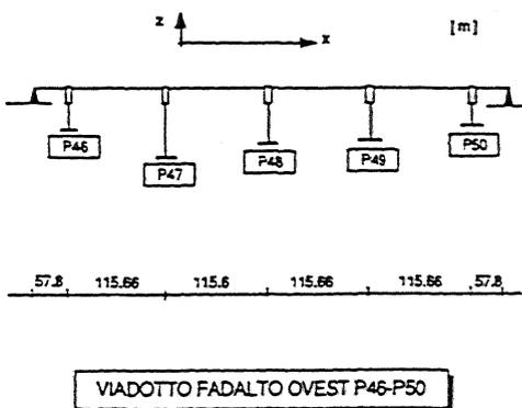
Fig.1. Schematic view of Fadalto viaduct
