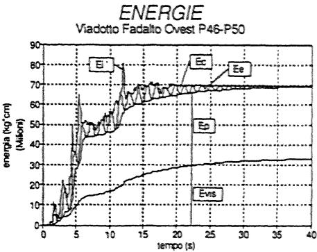
Fig. 9. Various types of energies vs time
