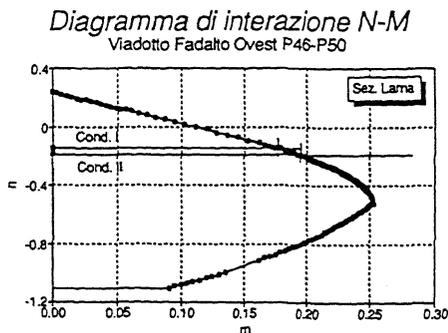
Fig.4 a,b M-N interaction diagrams for piers and walls
