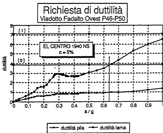
Fig. 7 Ductility demand for piers and walls vs ground acceleration
