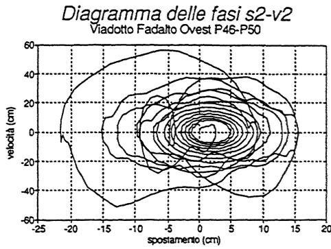
Fig. 6a,b Phase diagrams (velocity vs displacement) for the two degrees of freedom.
